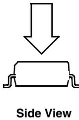
\* When positioned as shown, the Earth's gravity will result in a positive 1g output
