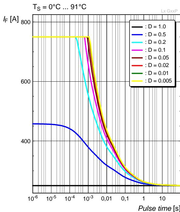
**Permissible Pulse Handling Capability****Zulässige Impulsbelastbarkeit  $I_F = f(t_p)$** D: Duty cycle,  $T_S = 85$  °C
