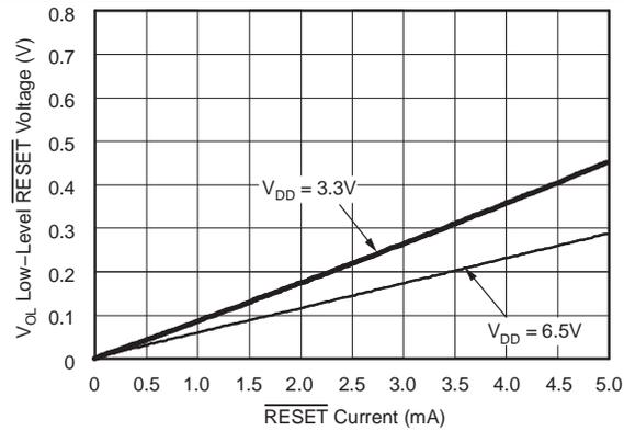
**Figure 8. Low-Level  $\overline{\text{RESET}}$  Voltage vs  $\overline{\text{RESET}}$  Current**
