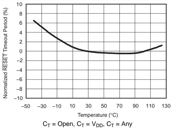
Figure 4. Normalized  $\overline{\text{RESET}}$  Timeout Period vs Temperature
