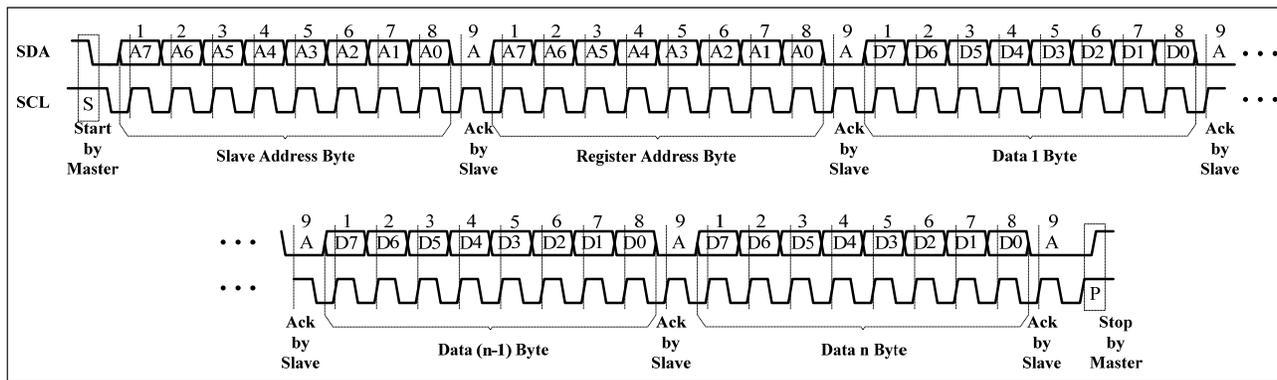
Figure 9 I2C Writing to IS31FL3748A (Automatic Address Increment)
