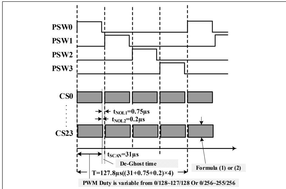
Figure 15 Scanning Timing
