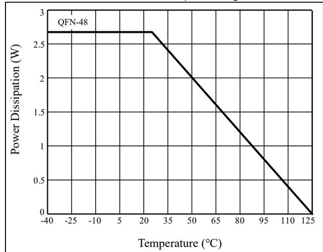
Figure 16 Dissipation Curve
