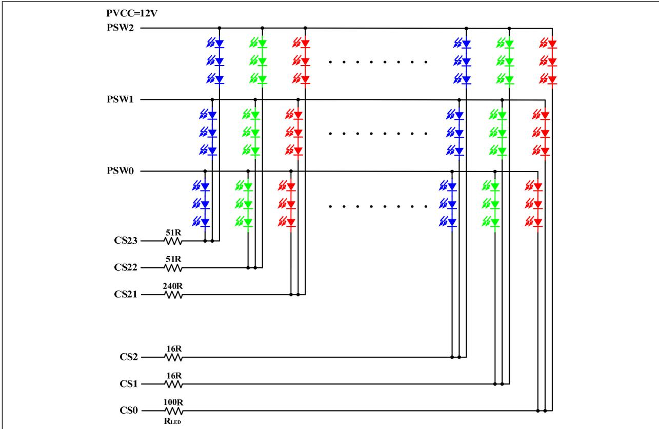
Figure 4 LED Circuit: 24x3
