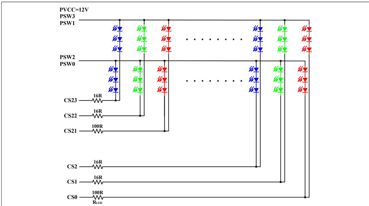
Figure 5 LED Circuit: 24x3
