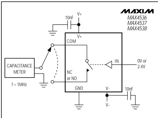
Figure 6. Channel-Off Capacitance
