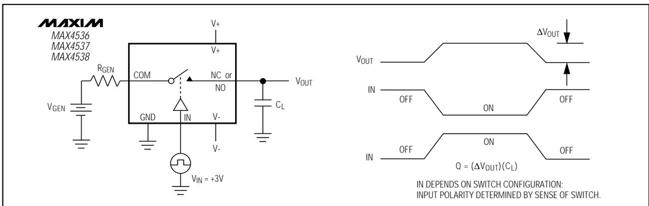
Figure 3. Charge Injection
