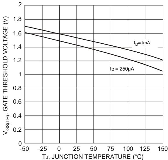
Fig. 5 Gate Threshold Variation vs. Junction Temperature
