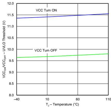
**Figure 3. UVLO Threshold vs. Temperature**
