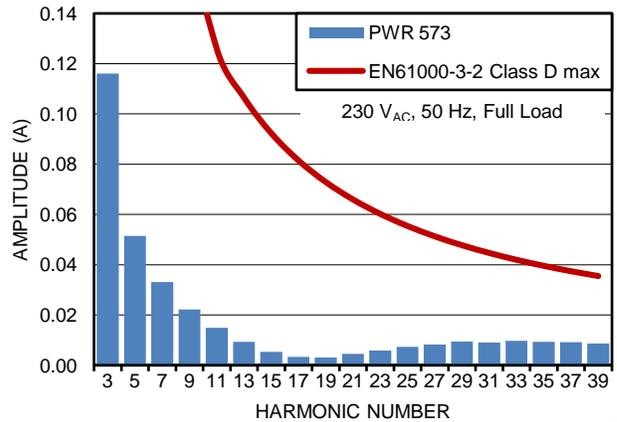
Figure 38. UCC28180EVM-573 Current Harmonics, (230-V<sub>AC</sub>, 50-Hz Input, Full Load, Without the Fundamental)
