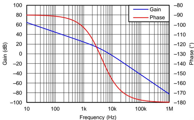
**Figure 32. Bode Plot of the Current Averaging Circuit**
