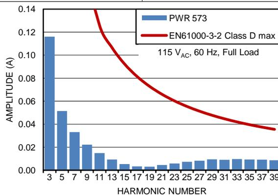
Figure 39. UCC28180EVM-573 Current Harmonics, (115-V<sub>AC</sub>, 60-Hz Input, Full Load, Without the Fundamental)
