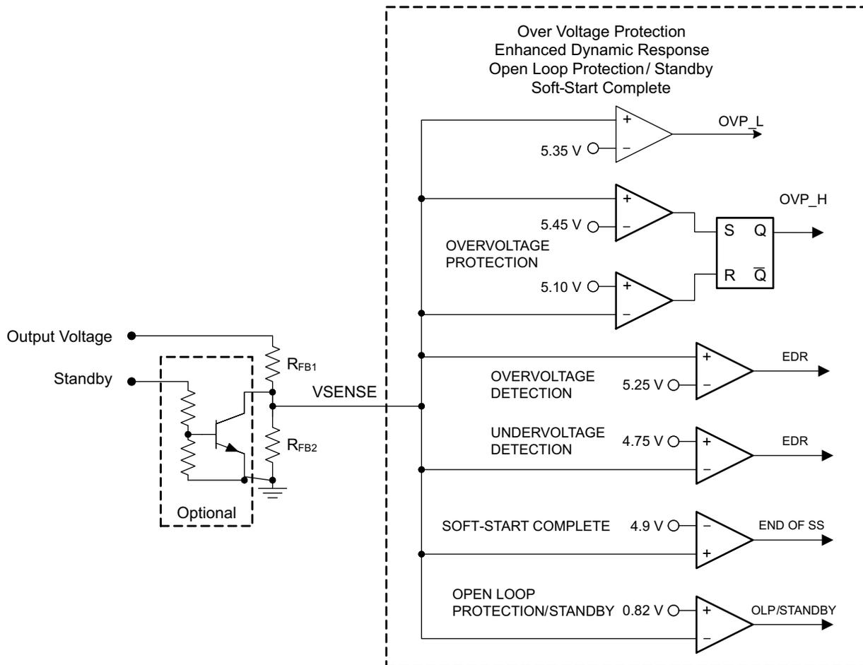
**Figure 25. OVP\_H, OVP\_L, EDR, OLP, Soft Start Complete**
