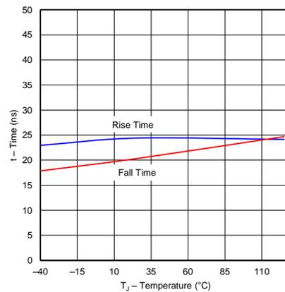
VCC = 15 V      C<sub>GATE</sub> = 4.7 nF      V<sub>GATE</sub> = 2 V-8 V
