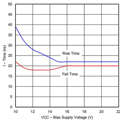
T<sub>J</sub> = 25 °C      C<sub>GATE</sub> = 4.7 nF      V<sub>GATE</sub> = 2 V-8 V
