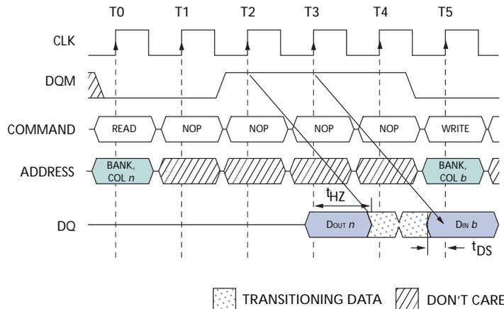
Notes: 1. CL = 3 is used for illustration; the READ command may be to any bank, and the WRITE command may be to any bank.
