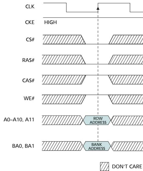
Figure 8: Meeting  $t_{RCD}$  (MIN) When  $2 < t_{RCD} (MIN)/t_{CK} \leq 3$
