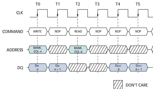
Notes: 1. CL = 2 is used for illustration; the WRITE command may be to any bank, and the READ command may be to any bank. DQM is LOW.
