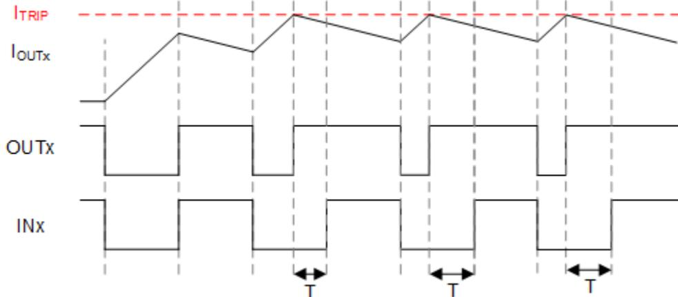
**Figure 7-6. Inductive Load Connected to VM, Cycle-by-cycle control, T has to be less than  $T_{OFF}$  of the DRV8955.**
