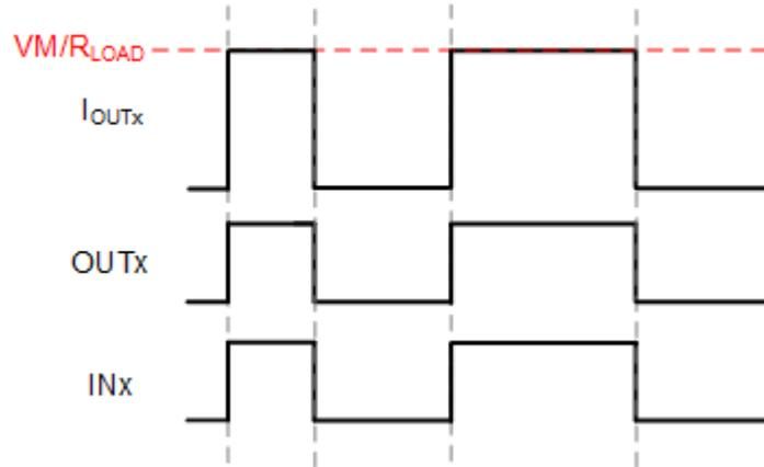
**Figure 7-8. Resistive Load Connected to ground, Cycle-by-cycle control**
