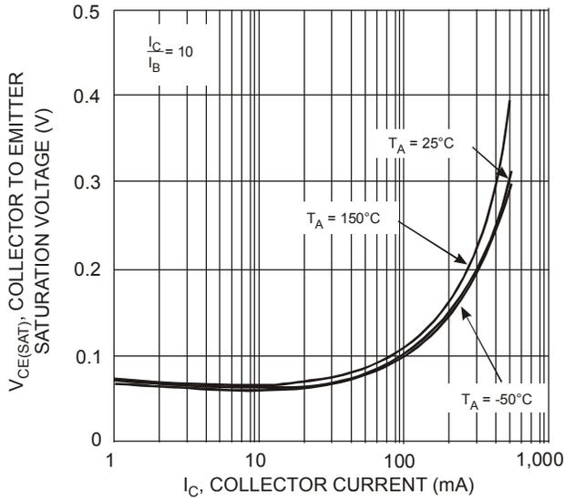
Fig. 5 Collector Emitter Saturation Voltage vs. Collector Current
