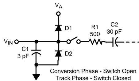
Figure 52. Equivalent Input Circuit
