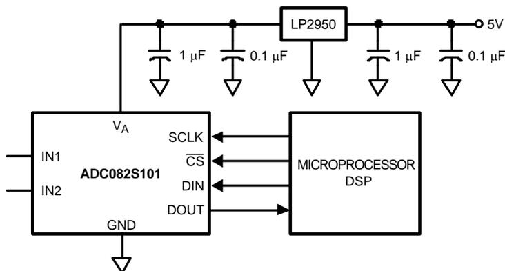
Figure 51. Typical Application Circuit
