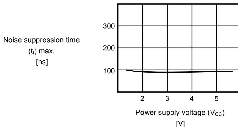
Figure 25 Noise Suppression Time for SDA Pin and SCL Pin
