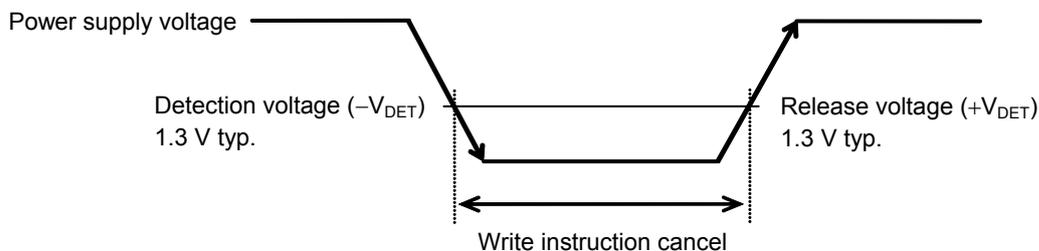
**Figure 23 Operation during Low Power Supply Voltage**
