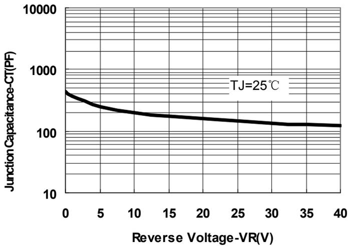
Fig.1-Typical Junction Capacitance
