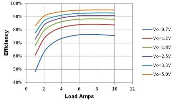
Figure 4 Efficiency vs. Load,  $V_{in} = 8\text{V}$ ,  $F_{sw} = 500\text{KHz}$
