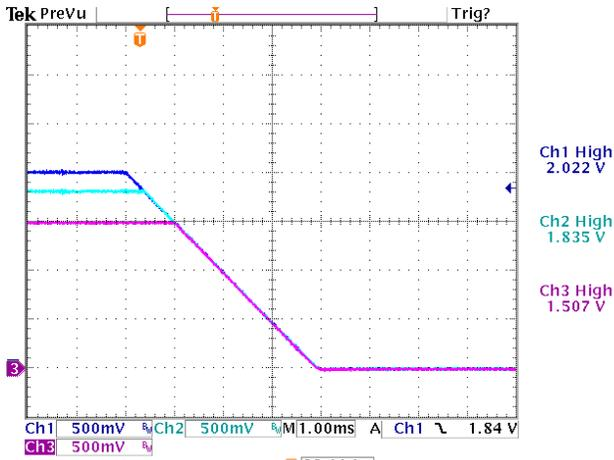
**Figure 22. Tracking Turn-Off. Falling Slew Rate is Programmed at 0.5V/ms.**
