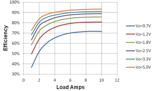
Figure 3. Efficiency vs. Load.  $V_{in} = 12\text{V}$ ,  $F_{sw} = 500\text{KHz}$
