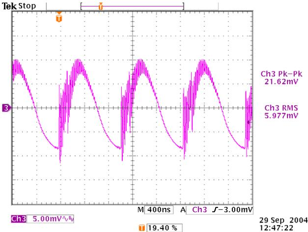
**Figure 41. Output Voltage Noise, Full Load, No Interleave**
