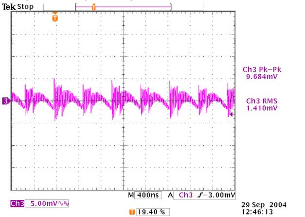
**Figure 42. Output Voltage Noise, Full Load, 180° Interleave**
