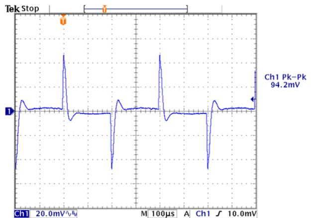
**Figure 10 Transient Response with Regulation set to 0 mV/A.**
