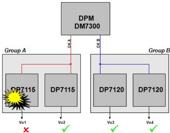
**Figure 32. No Group Fault Propagation**
