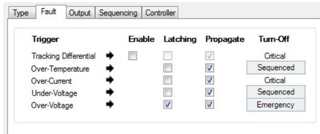
**Figure 27. GUI dPOL Fault Propagation Option Window**
