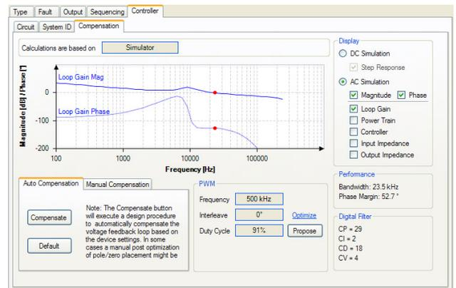
**Figure 37. PWM Controller Window**
