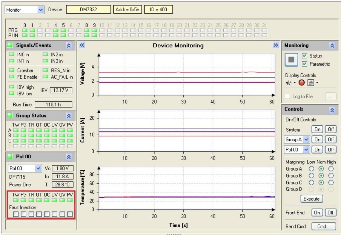
Figure 48. Fault Injection Controls In Monitor Window
