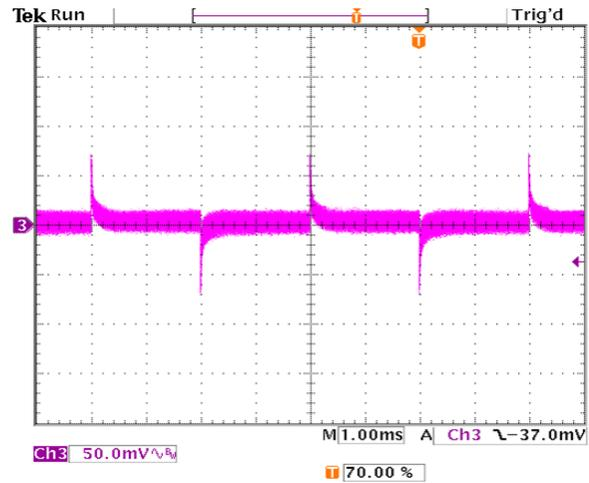
**Figure 44. Transient Response with Regulation set to 0.0 mV/A.**
