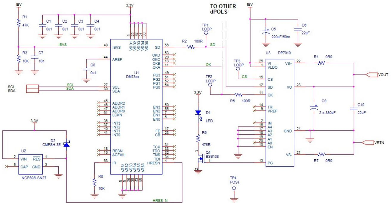
Figure 51. Typical Application with Digital Power Manager and I<sup>2</sup>C Interface
