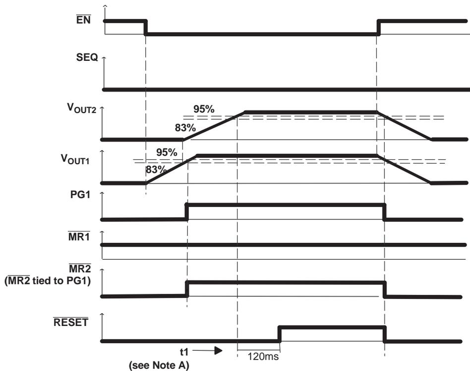
NOTE A:  $t_1$  – Time at which both  $V_{\text{OUT1}}$  and  $V_{\text{OUT2}}$  are greater than the PG1 thresholds and  $\overline{\text{MR1}}$  is logic high.
