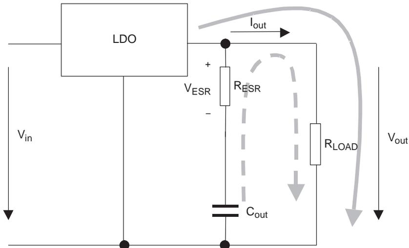
Figure 48. LDO Output Stage with Parasitic Resistances ESR
