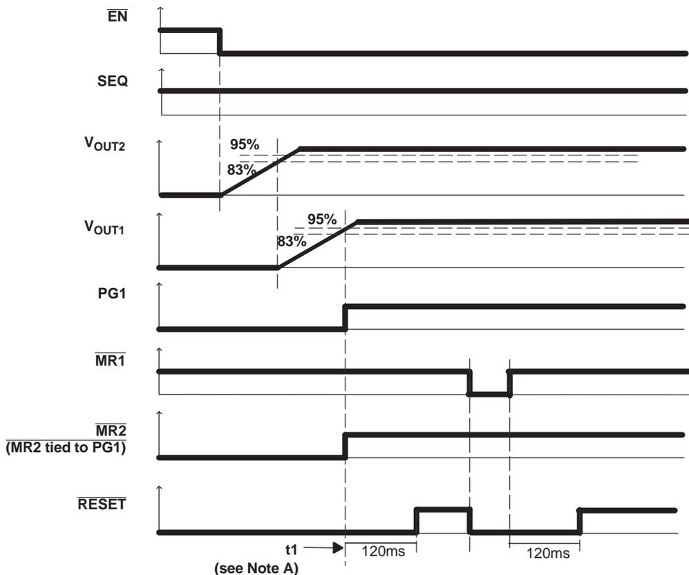
NOTE A:  $t_1$  – Time at which both  $V_{\text{OUT1}}$  and  $V_{\text{OUT2}}$  are greater than the PG1 thresholds and  $\overline{\text{MR1}}$  is logic high.
