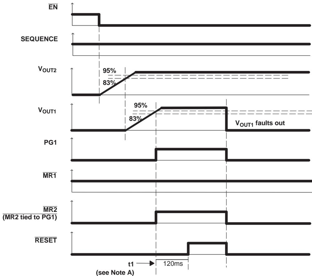
NOTE A:  $t_1$  – Time at which both  $V_{\text{OUT1}}$  and  $V_{\text{OUT2}}$  are greater than the PG1 thresholds and  $\overline{\text{MR1}}$  is logic high.
