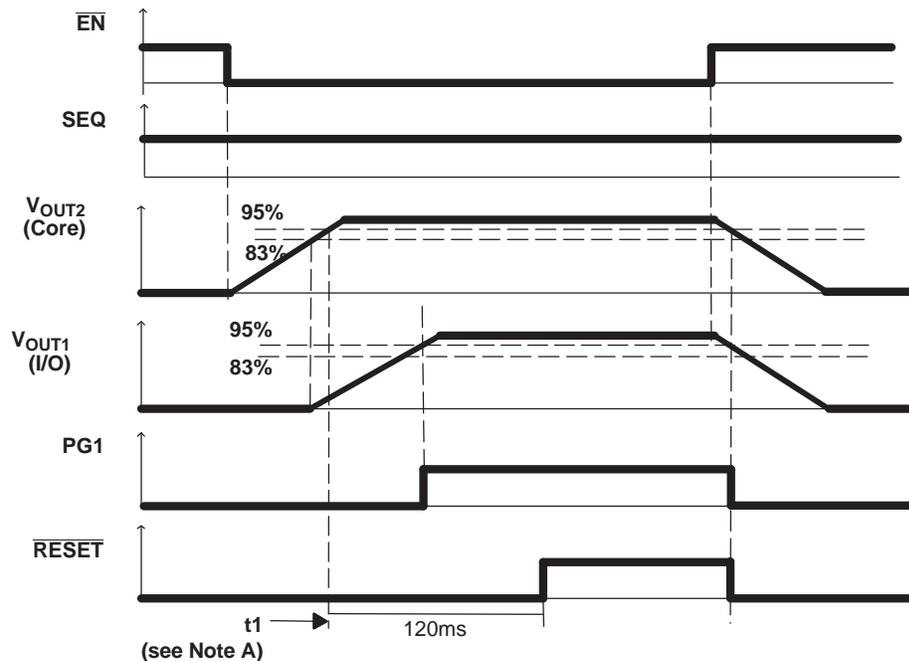
NOTE A:  $t_1$  – Time at which both  $V_{OUT1}$  and  $V_{OUT2}$  are greater than the PG1 thresholds and  $\overline{MR1}$  is logic high.
