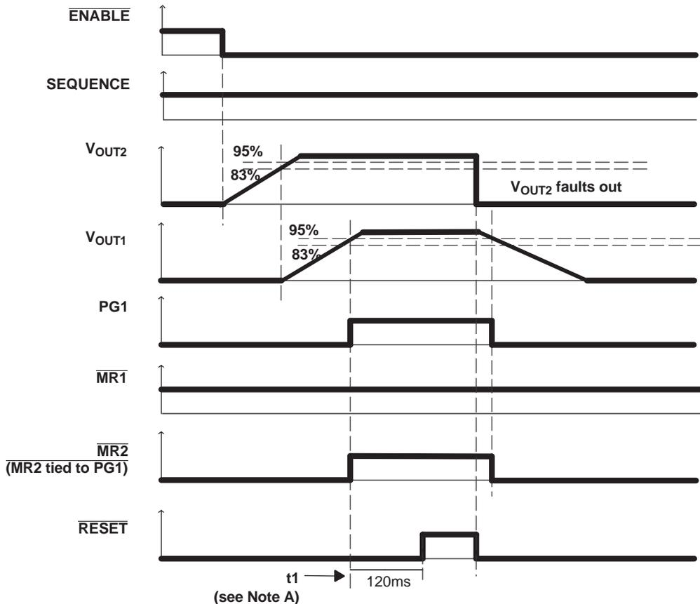
NOTE A:  $t_1$  – Time at which both  $V_{OUT1}$  and  $V_{OUT2}$  are greater than the PG1 thresholds and  $\overline{MR1}$  is logic high.
