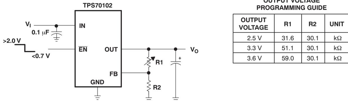
Figure 50. TPS70102 Adjustable LDO Regulator Programming
