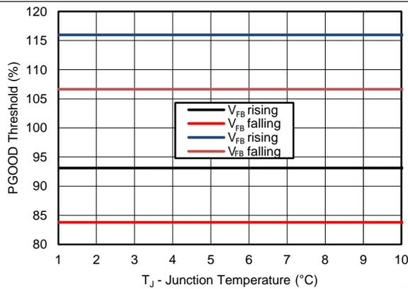
Figure 9. PGOOD Threshold vs Temperature
