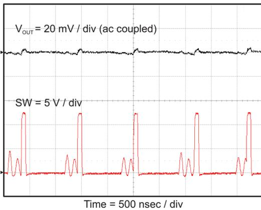
Figure 34. Output Voltage Ripple,  $I_{OUT} = 700 \text{ mA}$
