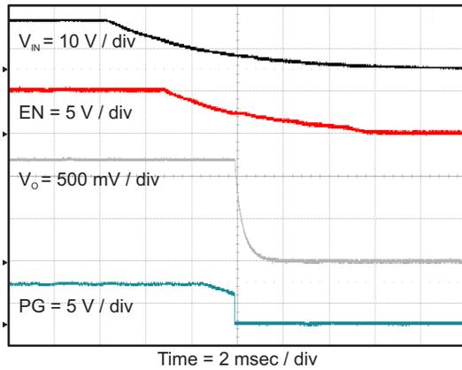
**Figure 38. Shut Down Relative to  $V_{IN}$  Falling**
