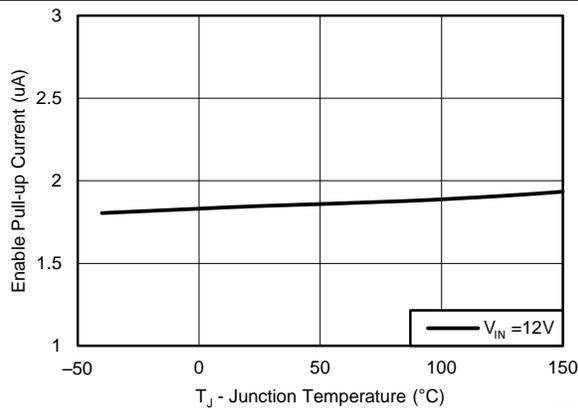
Figure 7. Enable Pull-Up Current, V<sub>EN</sub> = 1.0V
