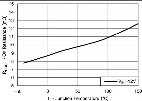
**Figure 5. Low-side R<sub>ds(on)</sub> vs Temperature**
