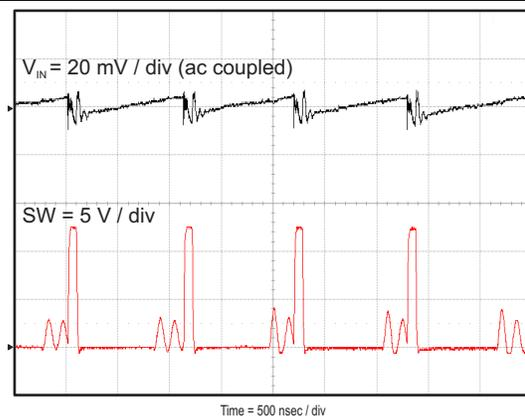
Figure 31. Input Voltage Ripple,  $I_{OUT} = 700\text{ mA}$
