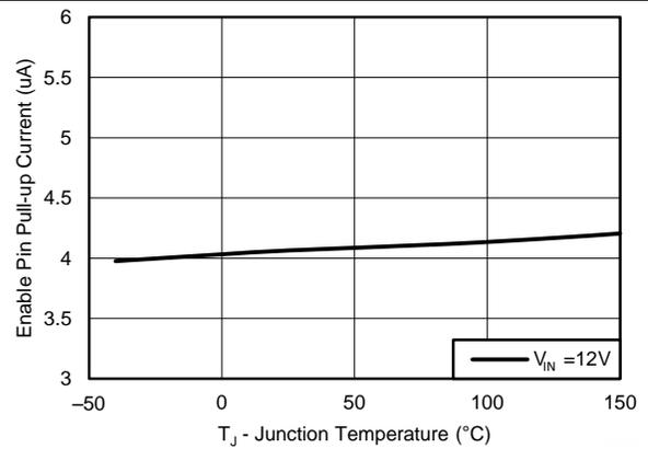
Figure 8. Enable Pull-Up Current, V<sub>EN</sub> = 1.3V
