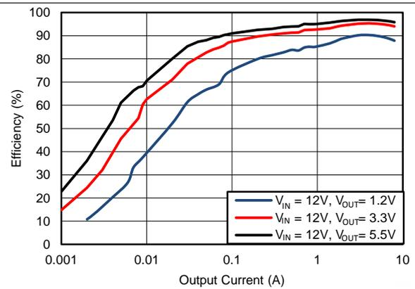
Figure 12. Efficiency, Mode = DCM, F<sub>SW</sub> = 400kHz
