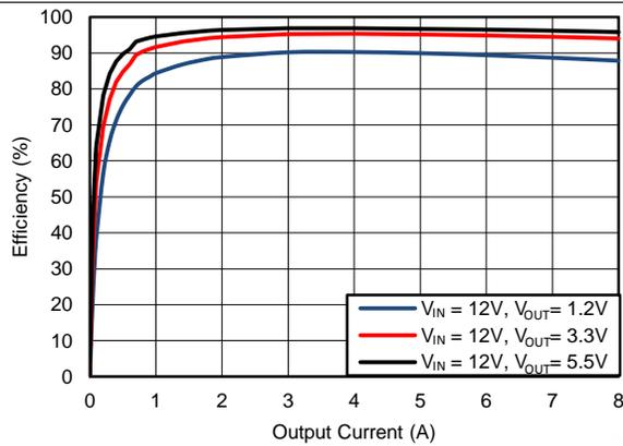
Figure 13. Efficiency, Mode = FCCM,  $F_{SW} = 400\text{kHz}$
