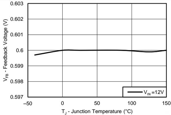
**Figure 3. Feedback Voltage vs Temperature**
