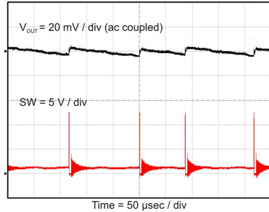
Figure 33. Output Voltage Ripple,  $I_{OUT} = 10 \text{ mA}$
