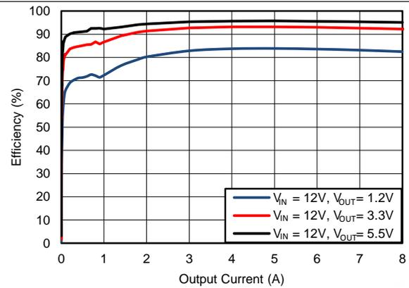
Figure 14. Efficiency, Mode = DCM,  $F_{SW} = 1200\text{kHz}$
