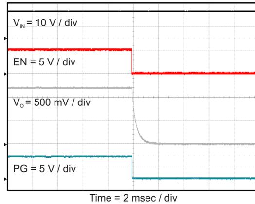
**Figure 39. Shut Down Relative to EN Falling**
