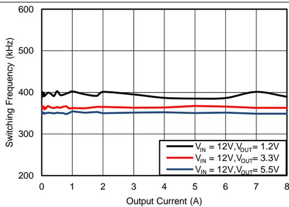
Figure 17.  $F_{SW}$  Load Regulation, Mode = FCCM,  $F_{SW} = 400\text{kHz}$
