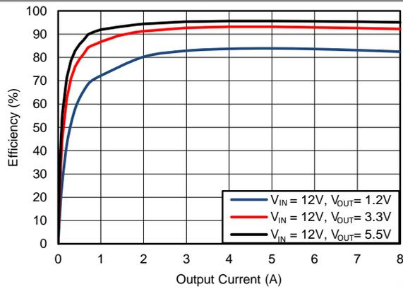
Figure 15. Efficiency, Mode = FCCM,  $F_{SW} = 1200\text{kHz}$
