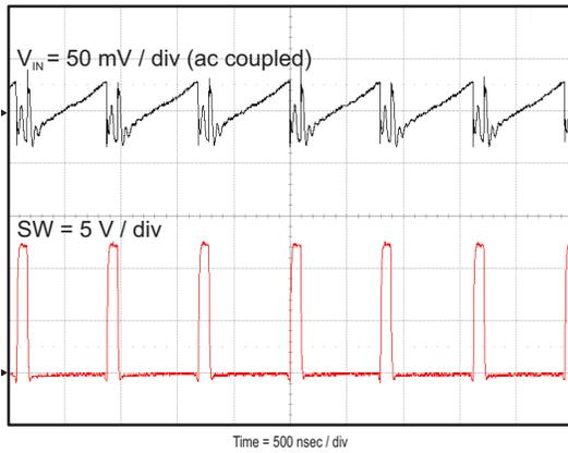
Figure 32. Input Voltage Ripple,  $I_{OUT} = 8 \text{ A}$
