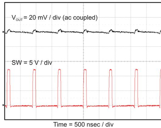
Figure 35. Output Voltage Ripple,  $I_{OUT} = 8 \text{ A}$
