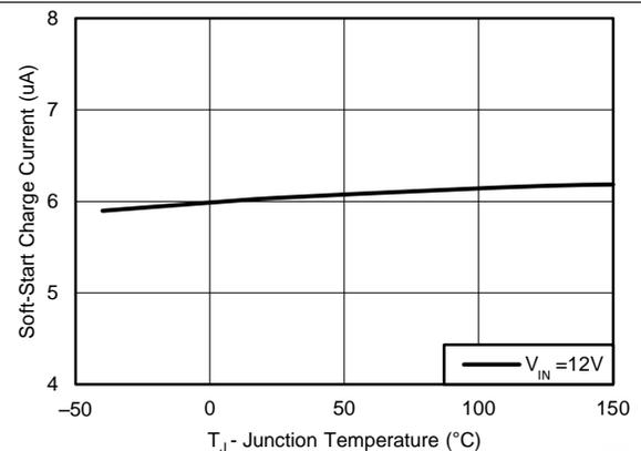
**Figure 6. Soft-Start Charge Current vs Temperature**
