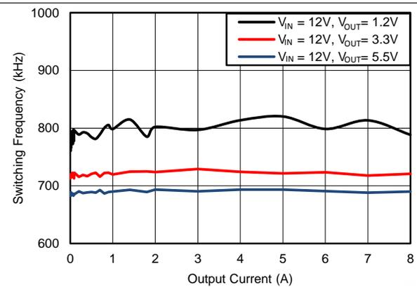
Figure 18.  $F_{SW}$  Load Regulation, Mode = FCCM,  $F_{SW} = 800\text{kHz}$
