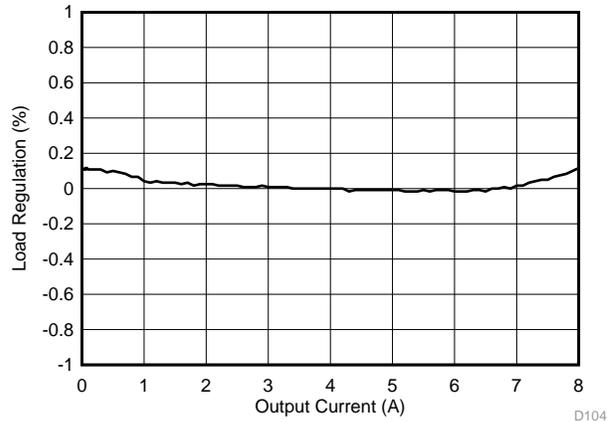
Figure 27. Load Regulation,  $V_{IN} = 12\text{ V}$
