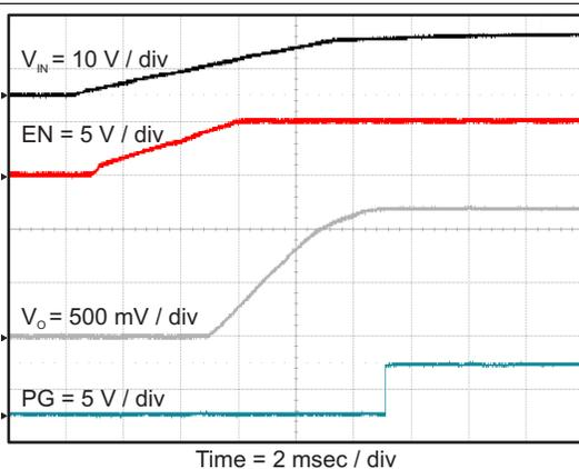
Figure 36. Start Up Relative to  $V_{IN}$  Rising
