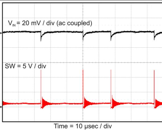
Figure 30. Input Voltage Ripple,  $I_{OUT} = 10\text{ mA}$
