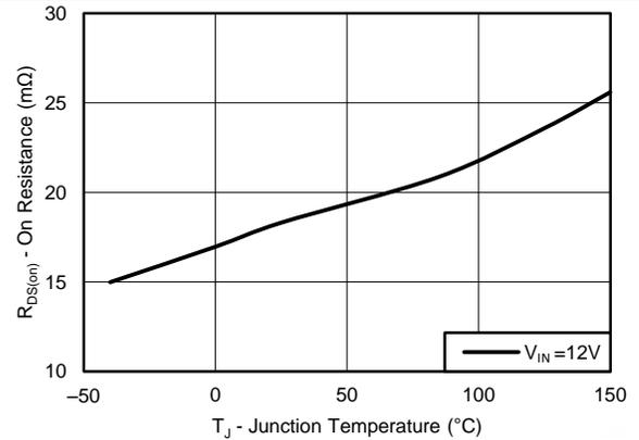
**Figure 4. High-side R<sub>ds(on)</sub> vs Temperature**
