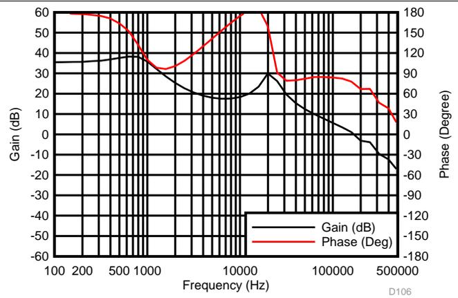
Figure 29. Loop Response,  $I_{OUT} = 6\text{ A}$
