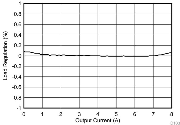
Figure 26. Load Regulation,  $V_{IN} = 5\text{ V}$
