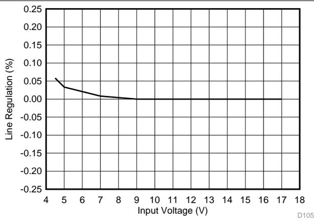
Figure 28. Line Regulation,  $I_{OUT} = 6\text{ A}$
