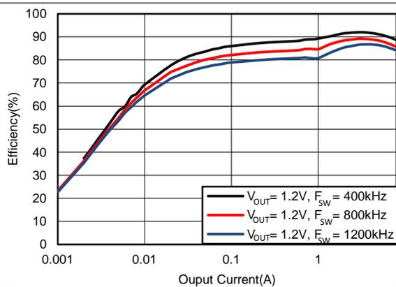
Figure 11. Efficiency with Internal VREG5 = 4.7 V, V<sub>IN</sub> = 12 V
