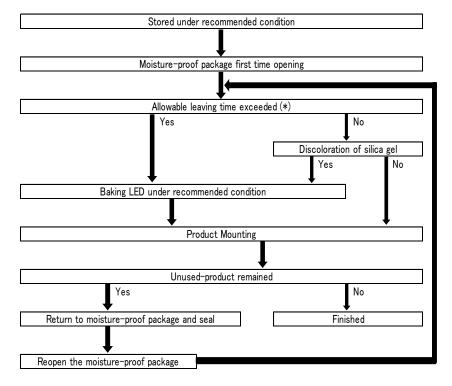
Allowable leaving time means the maximum allowable leaving time after opening package, which depends on each LED type.
