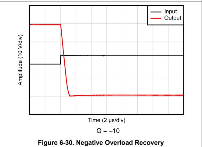
Figure 6-30. Negative Overload Recovery
