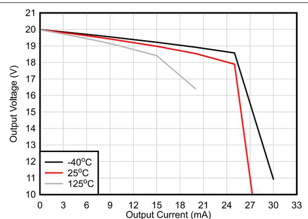
**Figure 6-12. Output Voltage Swing vs Output Current (Sourcing)**
