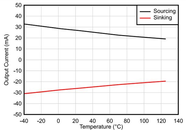
**Figure 6-36. Short-Circuit Current vs Temperature**
