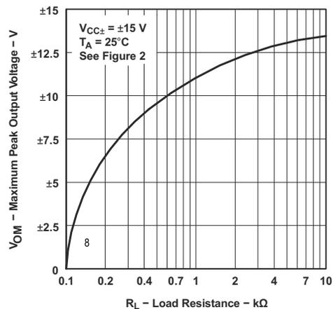
Figure 6-45. Maximum Peak Output Voltage vs Load Resistance
