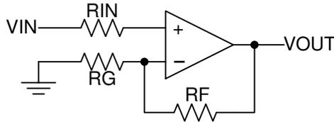
**Figure 9-11. Operational Amplifier Schematic for Noninverting Configuration**
