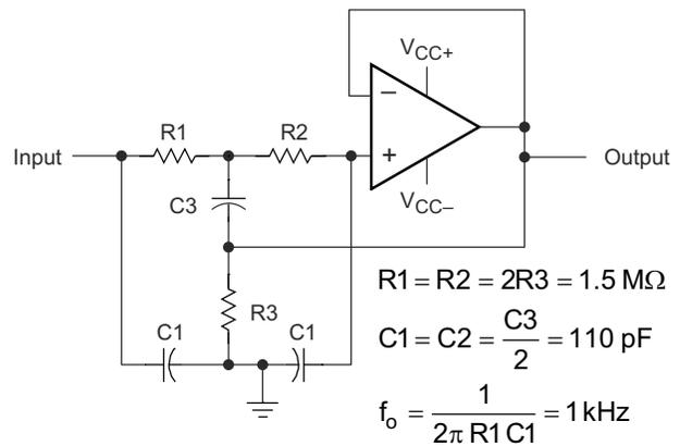
**Figure 9-7. High-Q Notch Filter**
