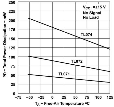
**Figure 6-53. Total Power Dissipation vs Free-Air Temperature**
