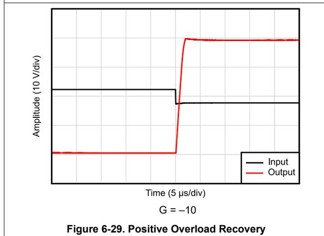
Figure 6-29. Positive Overload Recovery
