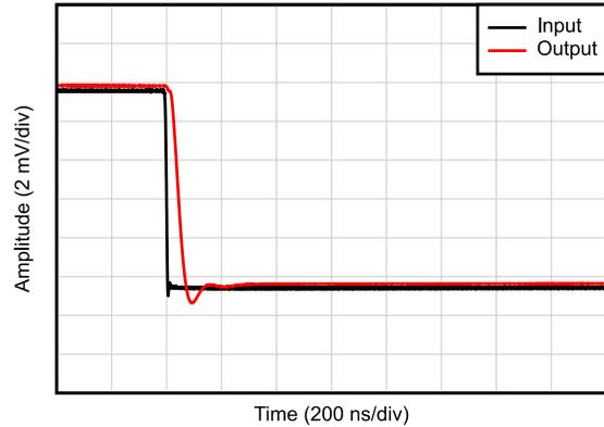
$C_L = 20\text{ pF}$ ,  $G = 1$ , 10-mV step response
