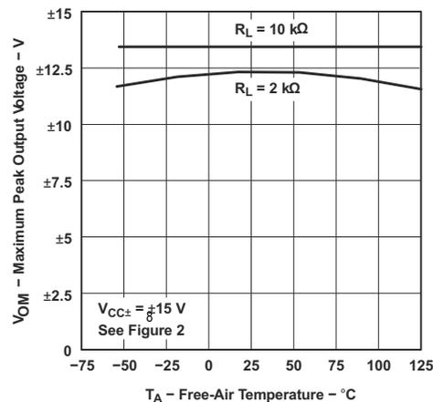
Figure 6-44. Maximum Peak Output Voltage vs Free-Air Temperature
