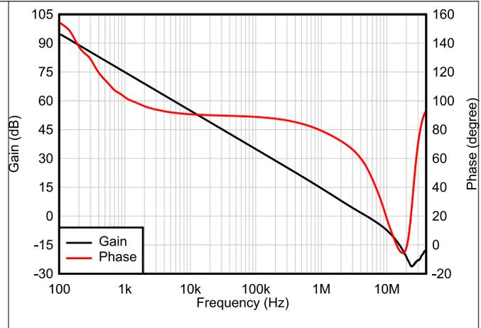
**Figure 6-8. Open-Loop Gain and Phase vs Frequency**
