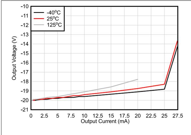
Figure 6-13. Output Voltage Swing vs Output Current (Sinking)
