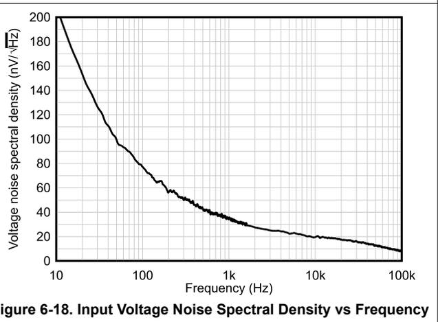
Figure 6-18. Input Voltage Noise Spectral Density vs Frequency
