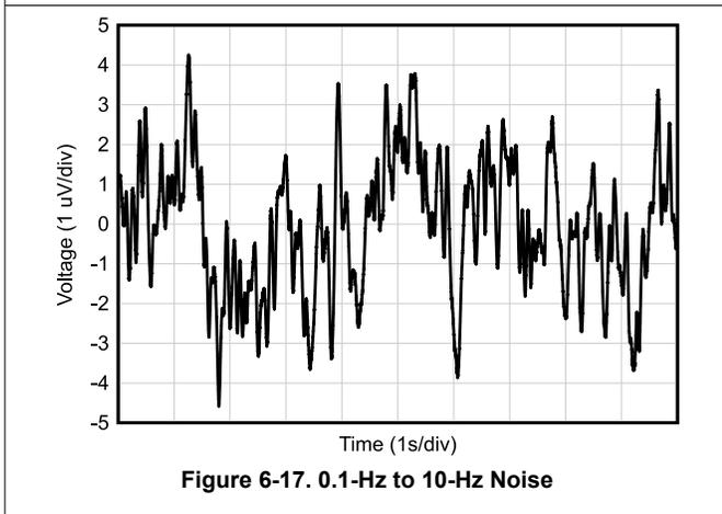
Figure 6-17. 0.1-Hz to 10-Hz Noise
