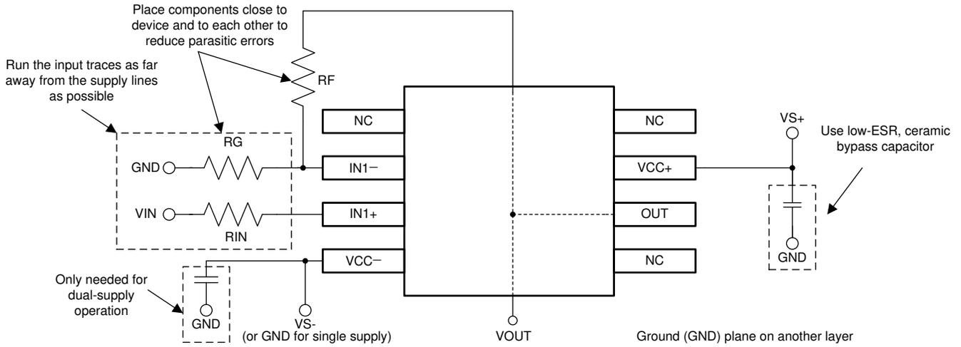
**Figure 9-10. Operational Amplifier Board Layout for Noninverting Configuration**
