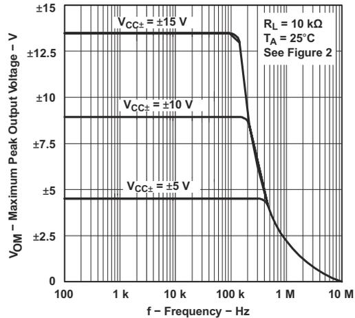
Figure 6-41. Maximum Peak Output Voltage vs Frequency
