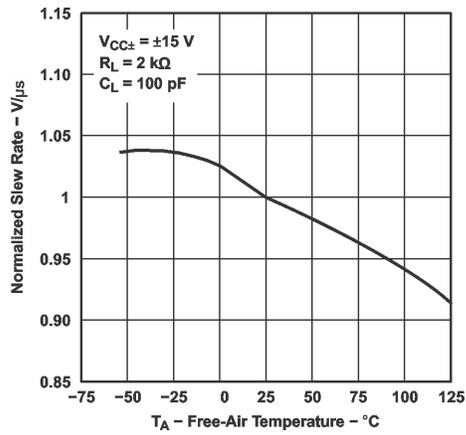
**Figure 6-54. Normalized Slew Rate vs Free-Air Temperature**
