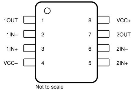
**Figure 5-5. TL072x D, DDF, JG, P, PS, and PW Package,
