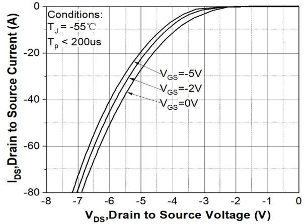
**Figure 8. Body Diode Characteristic at T<sub>J</sub> = -55 °C**
