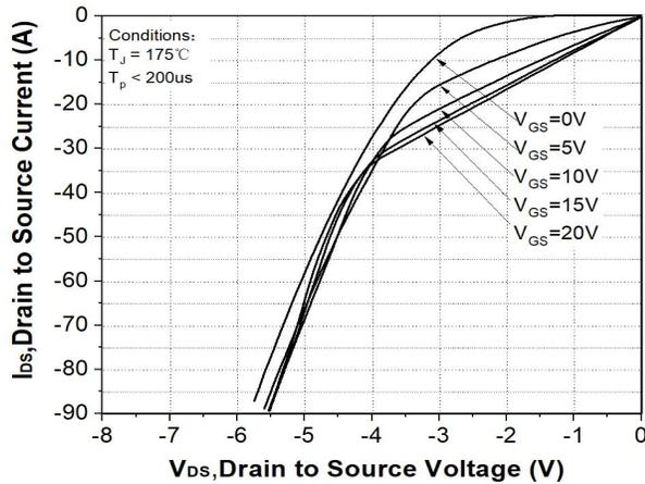
Figure 15. 3rd Quadrant Characteristic at  $T_J = 175^\circ\text{C}$
