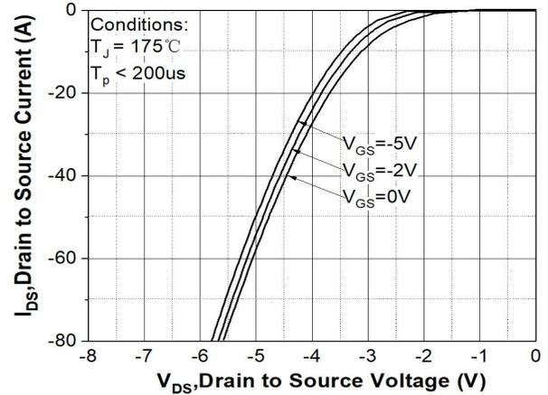
**Figure 10. Body Diode Characteristic at T<sub>J</sub> = 175 °C**
