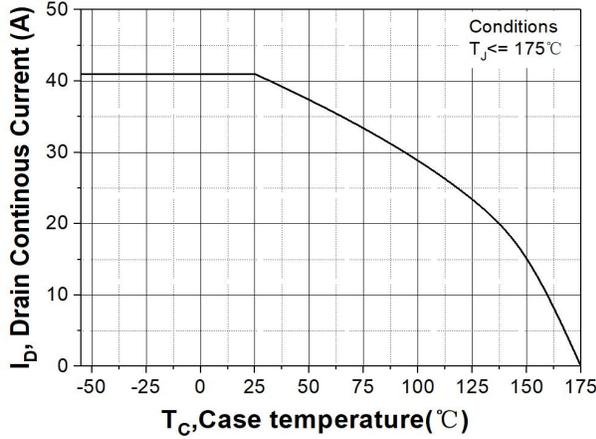
**Figure 19. Continuous Drain Current Derating vs. Case Temperature**
