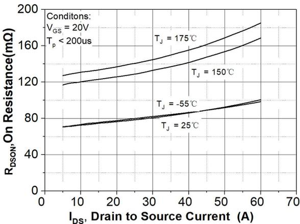
Figure 5. On-Resistance vs. Drain Current For Various Temperatures
