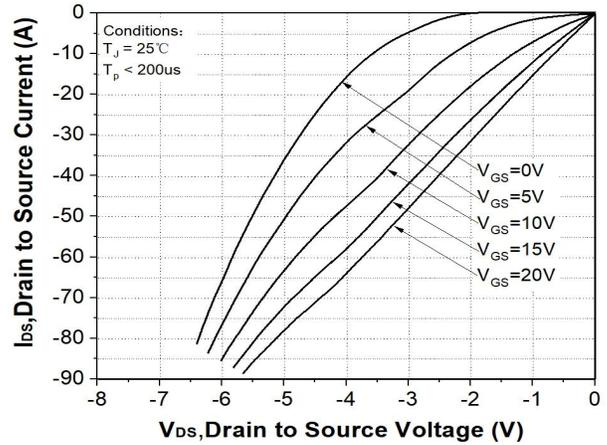
Figure 14. 3rd Quadrant Characteristic at  $T_J = 25^\circ\text{C}$
