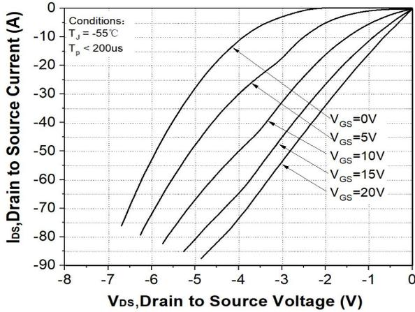
Figure 13. 3rd Quadrant Characteristic at  $T_J = -55^\circ\text{C}$
