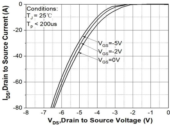
**Figure 9. Body Diode Characteristic at T<sub>J</sub> = 25 °C**
