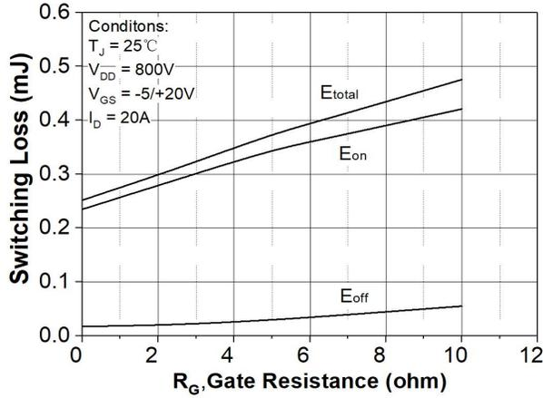
Figure 25. Clamped Inductive Switching Energy vs.  $R_{G(\text{ext})}$
