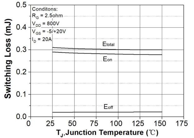
Figure 26. Clamped Inductive Switching Energy vs. Temperature
