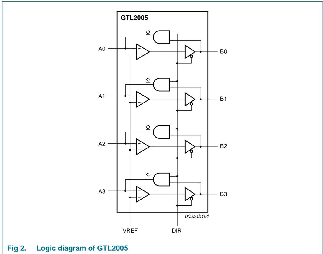
Fig 2. Logic diagram of GTL2005
