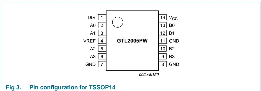
Fig 3. Pin configuration for TSSOP14
