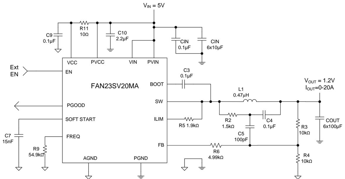
Figure 2. Typical Application with  $V_{IN} = 5\text{ V}$
