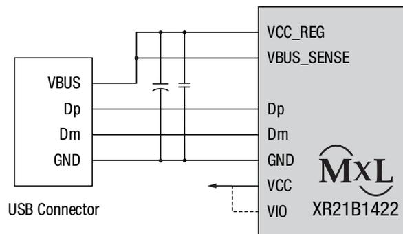
Figure 1: Bus-Powered Mode
