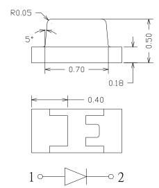
Units: mm / tolerance = +/-0.1mm
