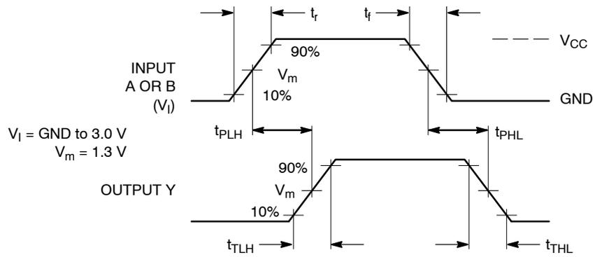
Figure 3. Switching Waveforms
