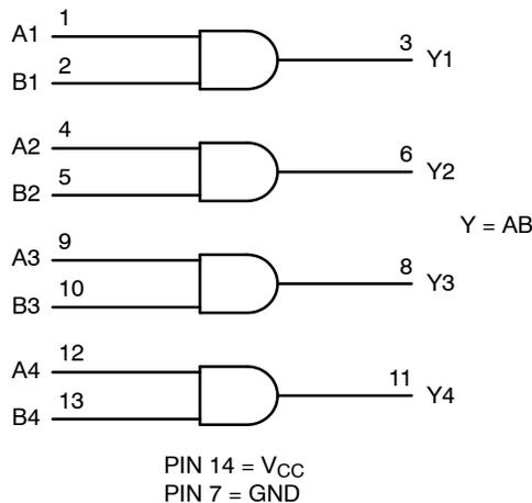
Figure 1. Logic Diagram
