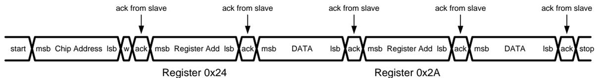
**Figure 74. Example Multi-Byte Command Sequencing**
