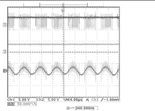
$V_{IN} = 3.6 \text{ V}$        $V_{OUT} = 3.3 \text{ V}$        $I_{LOAD} = 250 \text{ mA}$
