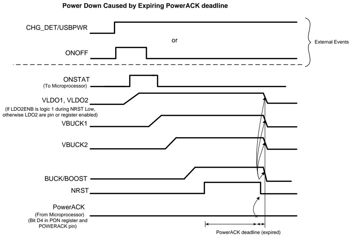
**Figure 68. Power Down Caused by Expiring PowerACK Deadline**
