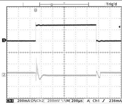
$V_{IN} = 4.2\text{ V}$        $V_{OUT} = 3.3\text{ V}$        $I_{LOAD} = 0\text{ to }500\text{ mA}$
