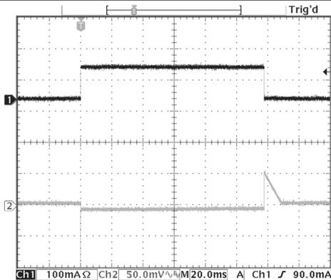
$V_{IN} = 3.6\text{ V}$        $V_{OUT} = 3.3\text{ V}$       Load = 0 to 100 mA
