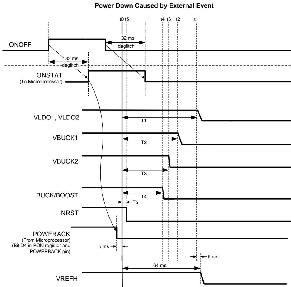
**Figure 67. Power-Down Event Caused by External Event**
