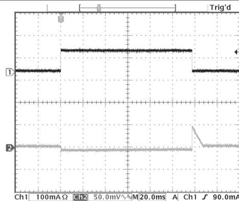
$V_{IN} = 3.6\text{ V}$        $V_{OUT} = 1.8\text{ V}$       Load = 0 to 100 mA
