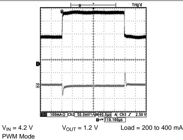
**Figure 27. Buck1 Load Transient Response**
