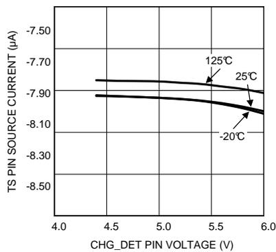
Figure 3. TS Pin Current vs CHG\_DET
