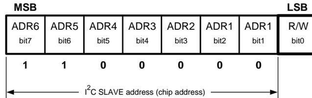
Figure 71. I<sup>2</sup>C Chip Address
