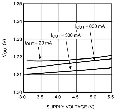
$V_{OUT} = 1.2 \text{ V}$
