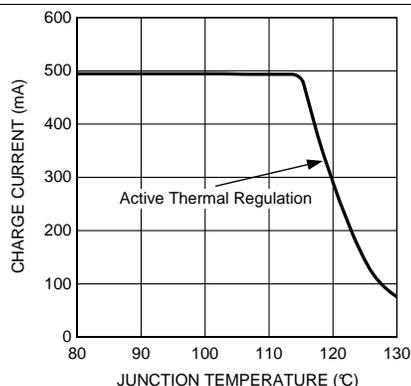
Figure 10. Thermal Regulation of Charge Current
