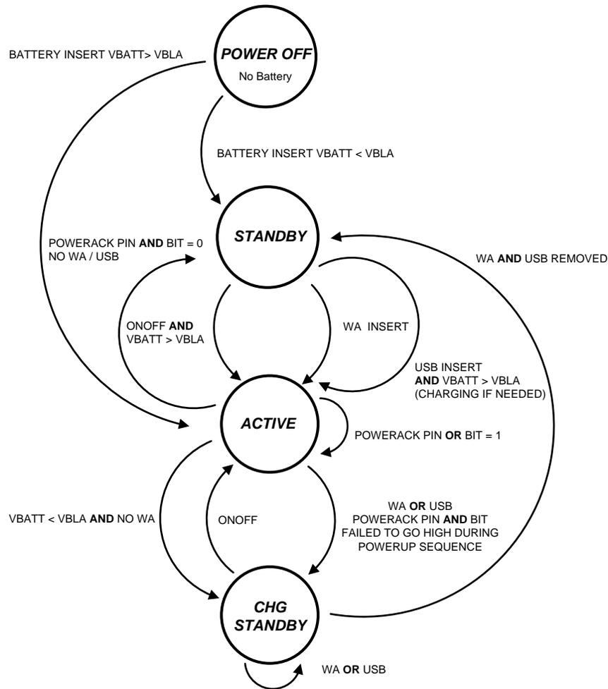
Figure 64. Operating Mode State Diagram
