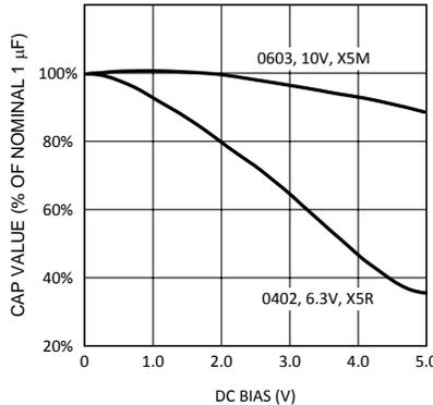
**Figure 76. Typical Variation in Capacitance vs DC Bias**
