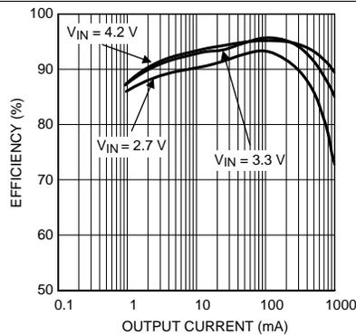
$V_{OUT} = 3.3 \text{ V}$
