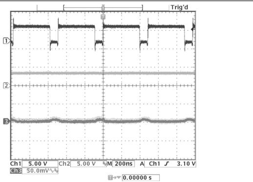
$V_{IN} = 4.2 \text{ V}$        $V_{OUT} = 3.3 \text{ V}$        $I_{LOAD} = 250 \text{ mA}$
