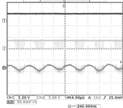
$V_{IN} = 3.35\text{ V}$        $V_{OUT} = 3.3\text{ V}$        $I_{LOAD} = 250\text{ mA}$
