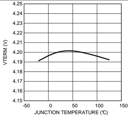
Figure 1. V<sub>TERM</sub> 4.2 V vs Temperature
