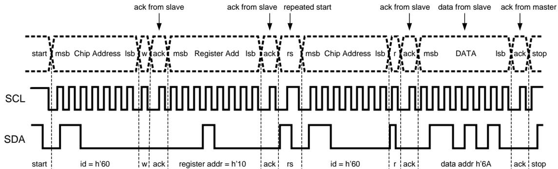
Figure 73. I<sup>2</sup>C Read Cycle
