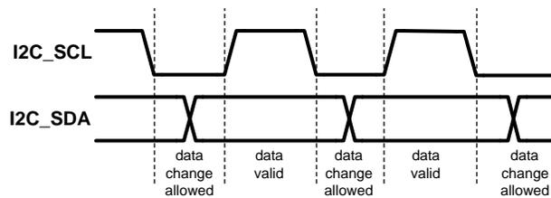
Figure 69. I<sup>2</sup>C Data Valid Diagram
