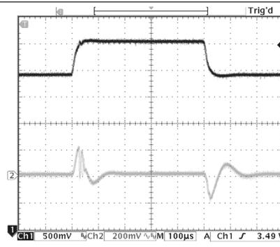
$V_{IN} = 3\text{ V to }3.6\text{ V}$        $V_{OUT} = 3.3\text{ V}$        $I_{LOAD} = 500\text{ mA}$
