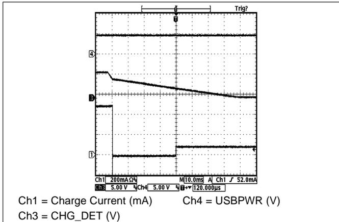
Figure 77. Wall Adapter Removal With USBPWR Present
