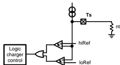
Figure 56. Battery Temperature Monitor with TS Pin
