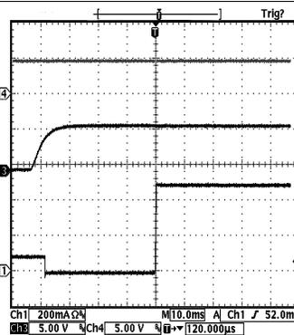
Ch1 = Charge Current (mA) Ch4 = USBPWR (V)
