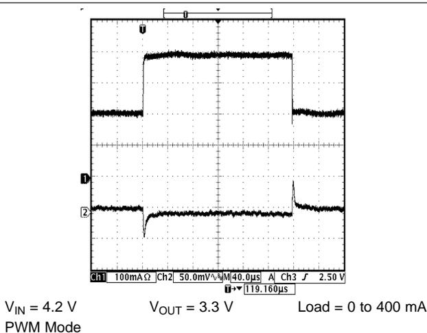
**Figure 29. Buck2 Load Transient Response**
