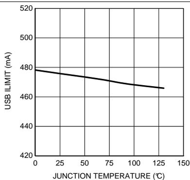
Figure 11. USB I<sub>LIMIT</sub> vs Temperature
