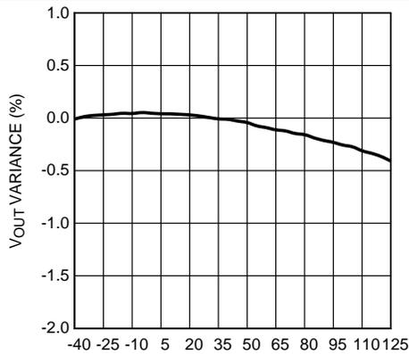
$V_{IN} = 4.3\text{ V}$        $V_{OUT} = 3.3\text{ V}$       Load = 100 mA
