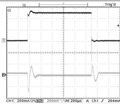
$V_{IN} = 2.7\text{ V}$        $V_{OUT} = 3.3\text{ V}$        $I_{LOAD} = 0\text{ to }500\text{ mA}$
