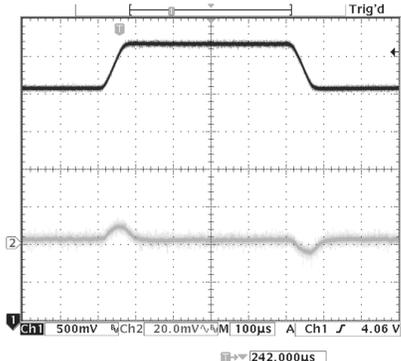
$V_{IN} = 3.6\text{ to }4.5\text{ V}$        $V_{OUT} = 3.3\text{ V}$       Load = 150 mA
