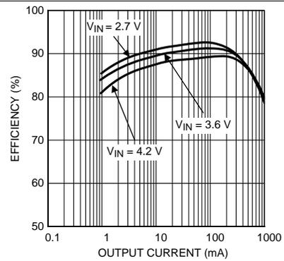
$V_{OUT} = 1.8 \text{ V}$
