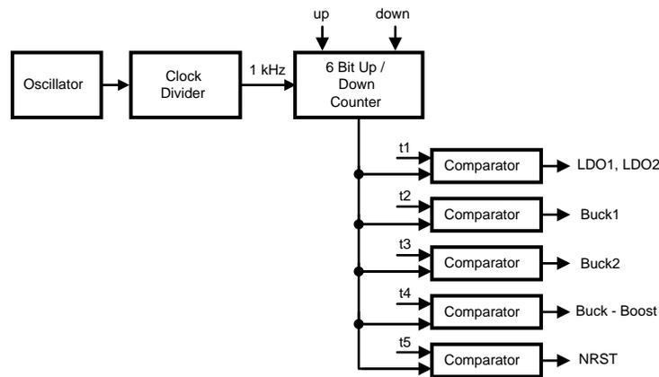
Figure 66. Power Sequencer Block Diagram
