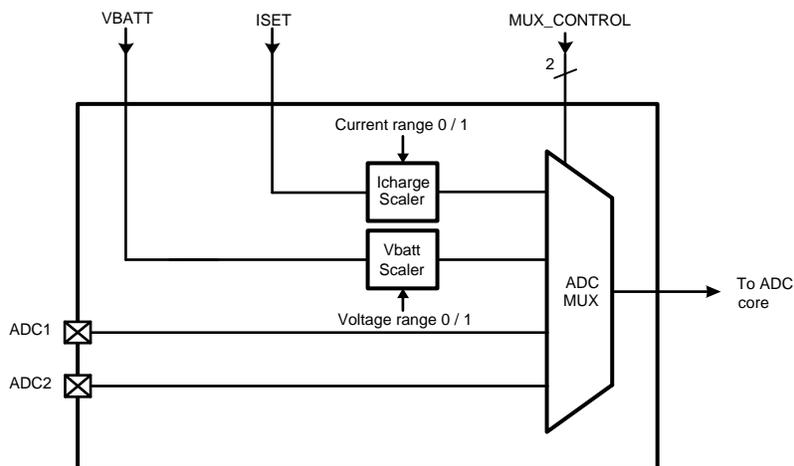
**Figure 59. ADC Analog Front-End Block Diagram**
