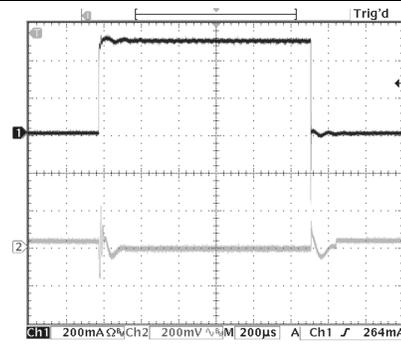
$V_{IN} = 3.6\text{ V}$        $V_{OUT} = 3.3\text{ V}$        $I_{LOAD} = 0\text{ to }500\text{ mA}$
