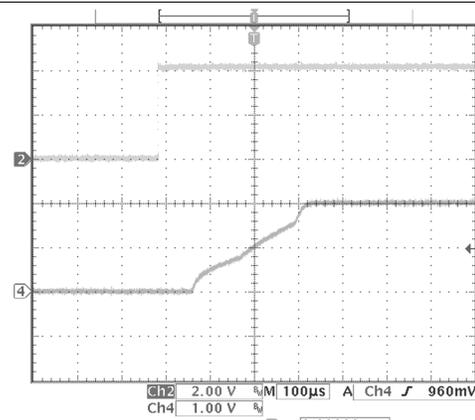
$V_{OUT} = 3.3 \text{ V}$       Load = 30 mA
