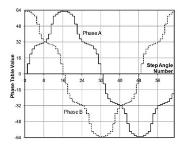
Figure 16: Resulting Example Current Profile
