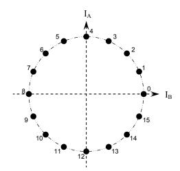
Figure A6: Phase Diagram for Quarter Step
