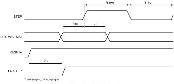
Figure 2: Control Input Interface Timing Diagram
