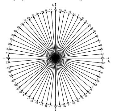
Figure 6: A3981 Phase Current Table as a Phase Diagram
