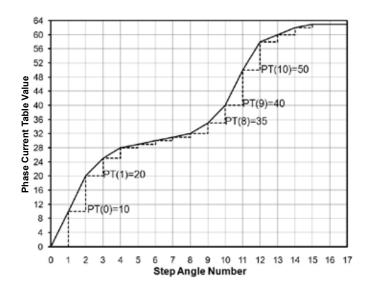
Figure 15: Digitizing the Example Current Profile
