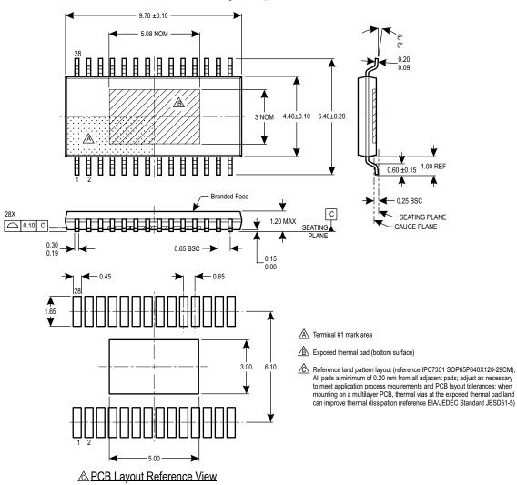
Figure 20: Package LP, 28-Pin TSSOP with Exposed Thermal Pad
