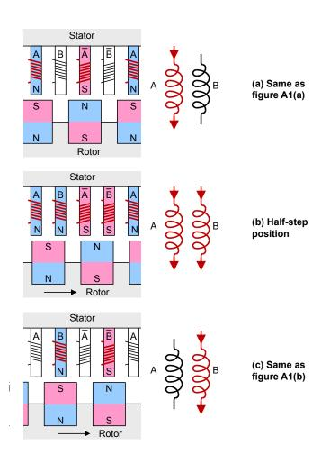
Figure A2: Half Step Operation
