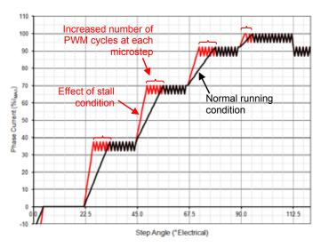
Figure 3. Effect of stall condition on current rise
