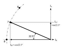
Figure A7: Calculating Phase Current Magnitudes
