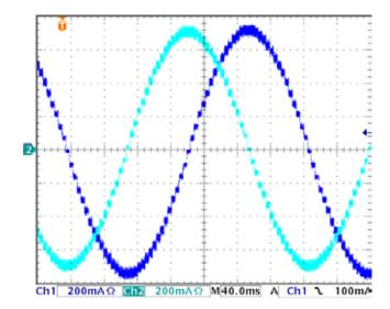
Figure A9: Measured Sixteenth-step Phase Current Sequence
