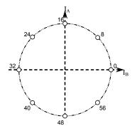
Figure 9: Half-step Phase Diagram Using STEP Input
