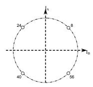
Figure 8: Full-step Phase Diagram Using STEP Input
