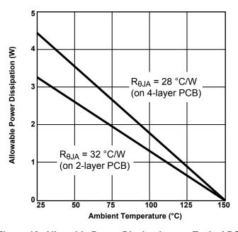
Figure 18: Allowable Power Dissipation, on Typical PCBs
