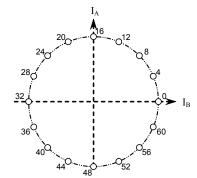
Figure 10: Quarter-step Phase Diagram Using STEP Input
