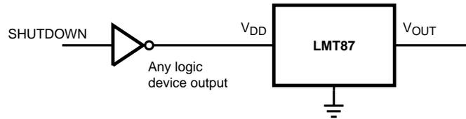
Figure 15. Simple Shutdown Connection of the LMT87
