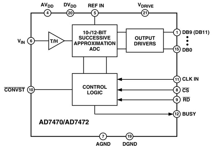
AD7470 IS A 10-BIT PART WITH DB0 TO DB9 AS OUTPUTS.
