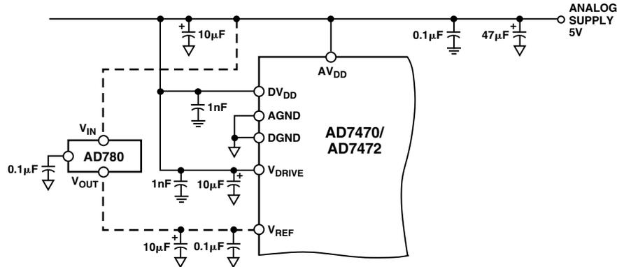
Figure 16. Decoupling Circuit
