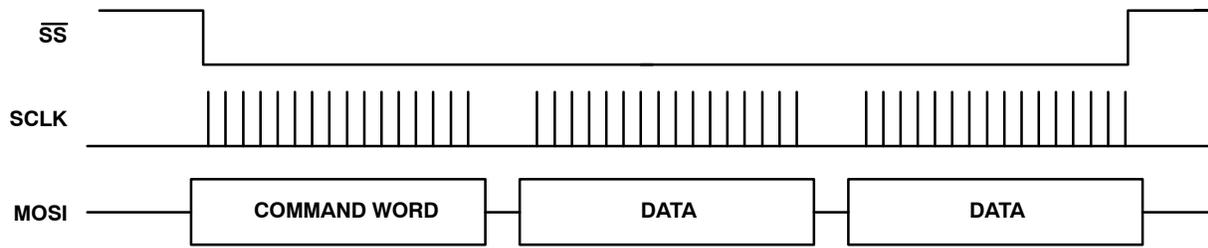
Figure 35. Write Operation for TSC2100 SPI Interface
