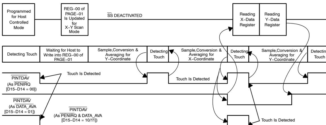
NOTE: If the  $\overline{\text{PINTDAV}}$  signal is programmed to be used for pen-interrupt by setting bits D15–D14 of REG01H/Page–2 to either 00, 01, or 11, then the high duration of  $\overline{\text{PINTDAV}}$  is given by:
