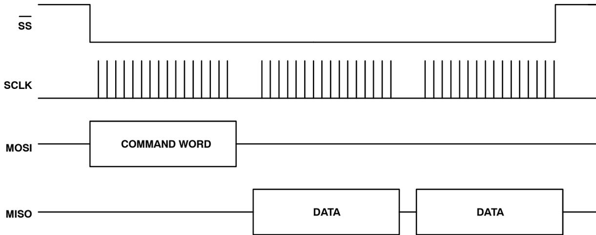
Figure 36. Read Operation for TSC2100 SPI Interface
