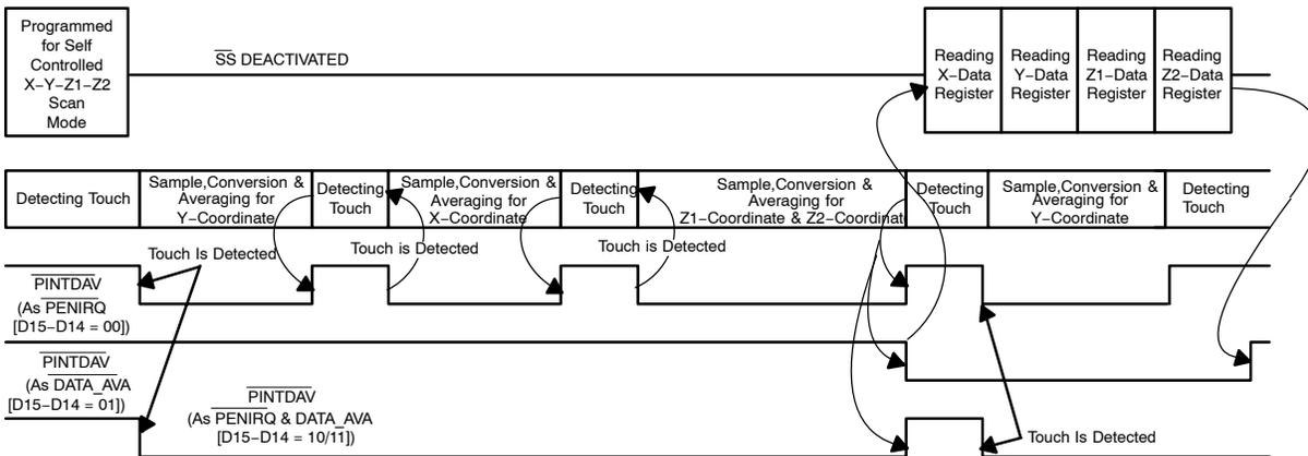
NOTE: If the PINTDAV signal is programmed to be used for pen-interrupt by setting bits D15–D14 of REG01H/Page–2 to either 00, 01, or 11, then the high duration of PINTDAV is given by:
