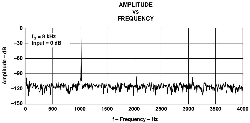
Figure 5-6. FFT-DAC Channel,  $f_s = 8$  kHz, Input = 0 dB
