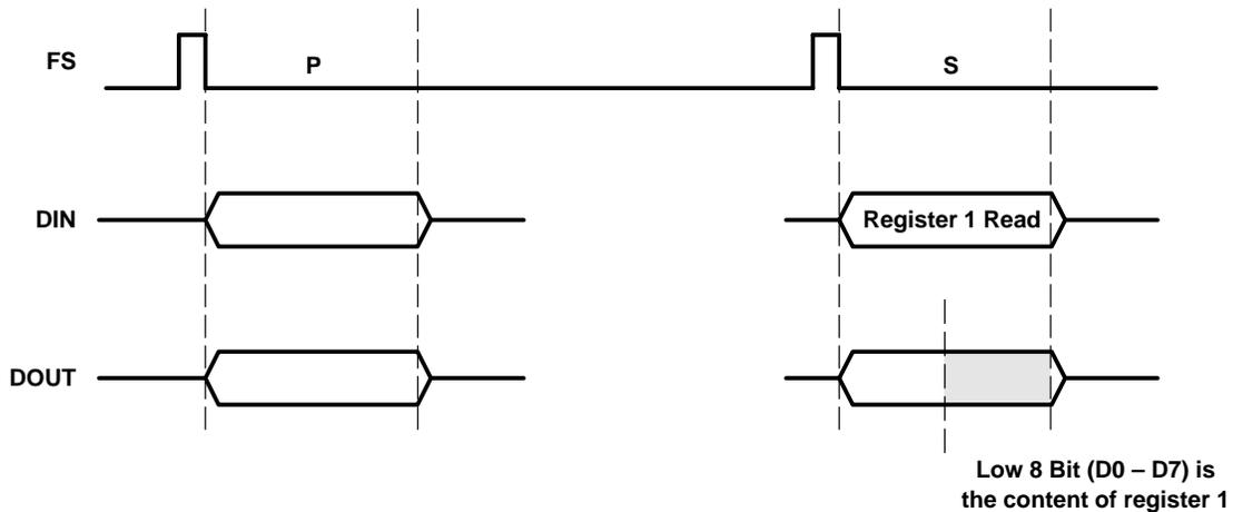
Figure 3–3. Device 3/Register 1 Read Operation Timing Diagram
