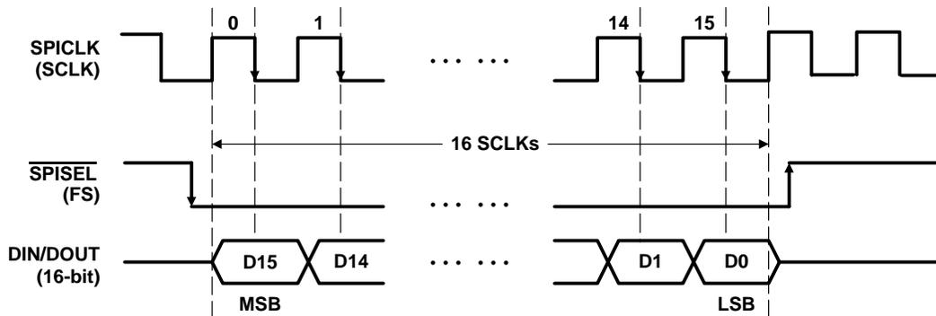
**Figure 2–10. Timing Diagram for the SPI\_CP0 Mode (M1M0 = 01)**
