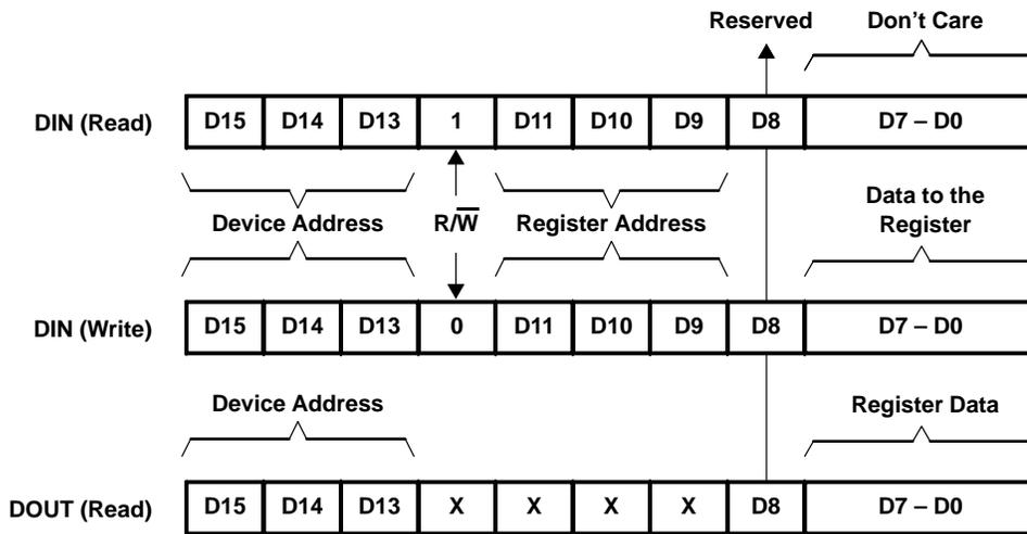
Figure 3-12. Secondary Communication DIN and DOUT Data Format
