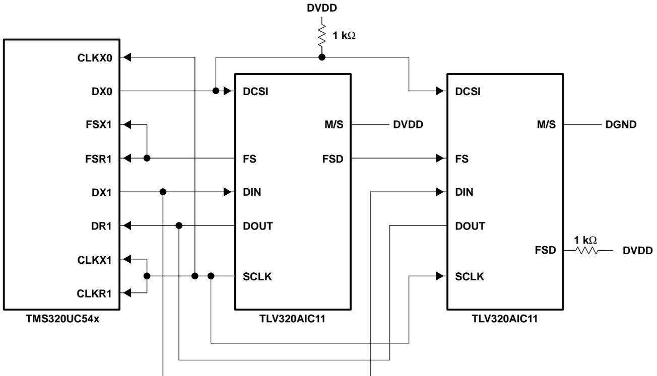
Figure 3–8. Direct Configuration
