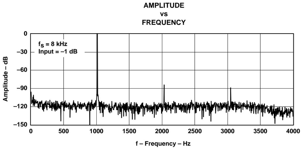
Figure 5-5. FFT-ADC Channel,  $f_s = 8$  kHz, Input = -1 dB
