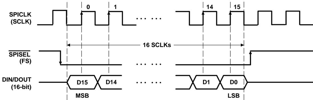
Figure 2–11. Timing Diagram for the SPI\_CP1 Mode (M1M0 = 10)
