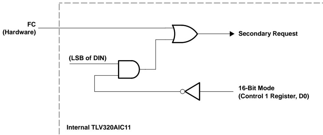
**Figure 3–2. Hardware and Software Secondary Communication Request**
