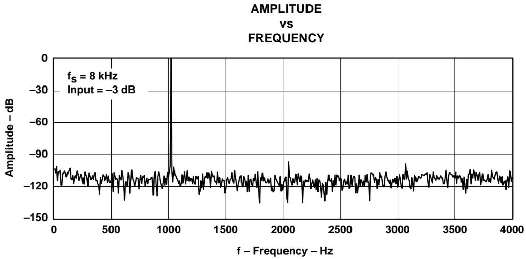
**Figure 5-4. FFT-DAC Channel,  $f_s = 8 \text{ kHz}$ , Input = -3 dB**
