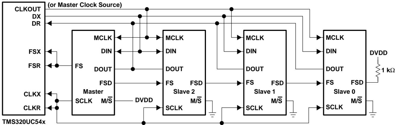
Figure 2–15. Cascade Mode Connection (to DSP Interface)
