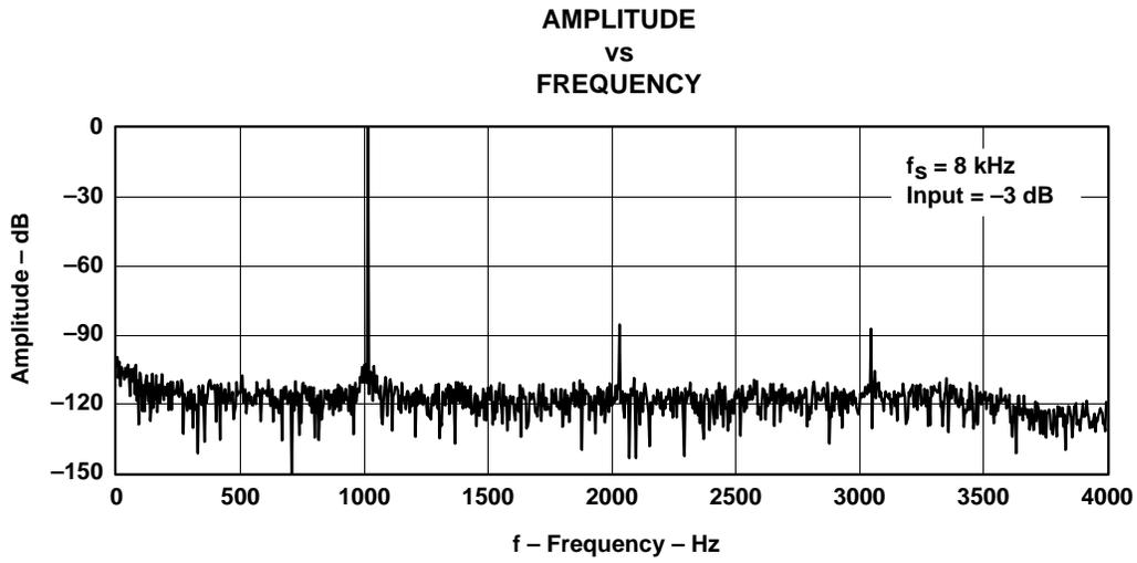
**Figure 5-3. FFT-ADC Channel,  $f_s = 8 \text{ kHz}$ , Input = -3 dB**
