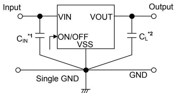
\*1.  $C_{IN}$  is a capacitor for stabilizing the input.
