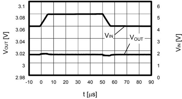
$I_{OUT} = 30\text{ mA}$ ,  $t_r = t_f = 5.0\ \mu\text{s}$ ,  $C_{OUT} = 4.7\ \mu\text{F}$ ,  $C_{IN} = 0\ \mu\text{F}$
