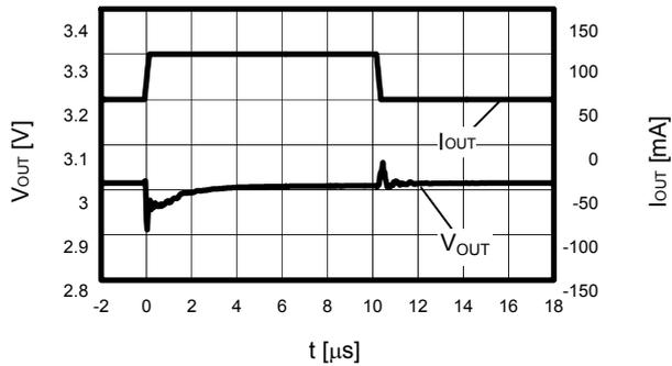
$V_{IN} = 4.0\text{ V}$ ,  $C_{OUT} = 4.7\ \mu\text{F}$ ,  $C_{IN} = 1.0\ \mu\text{F}$ ,
