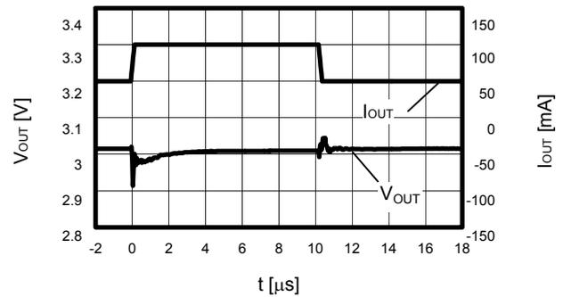
(3) ON/OFF pin transient response characteristics
