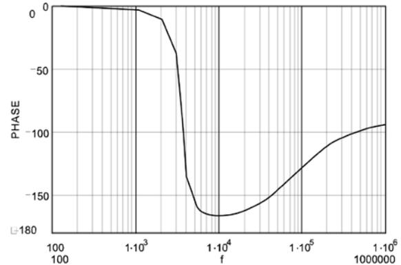
Figure 6. The Phase Curve with ESR = 0.002Ω
