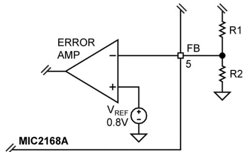
Figure 2. Voltage-Divider Configuration
