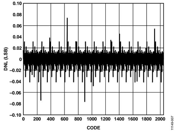
Figure 7. Typical DNL, 11 mA at 25°C
