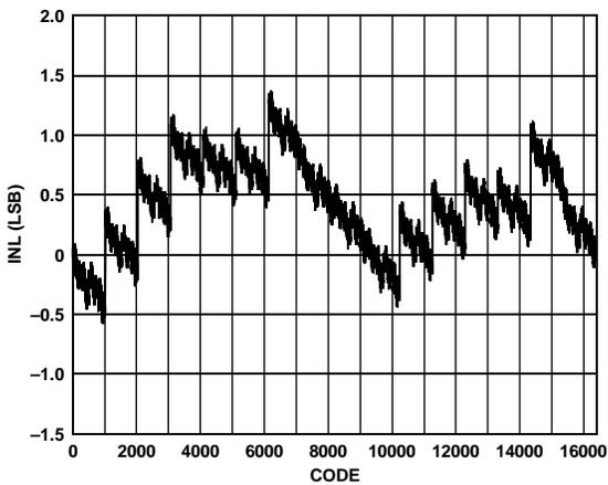
Figure 57. Typical INL, 22 mA at 25°C
