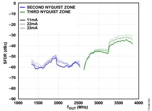
Figure 92. SFDR vs.  $f_{OUT}$  over DAC  $I_{OUTFS}$
