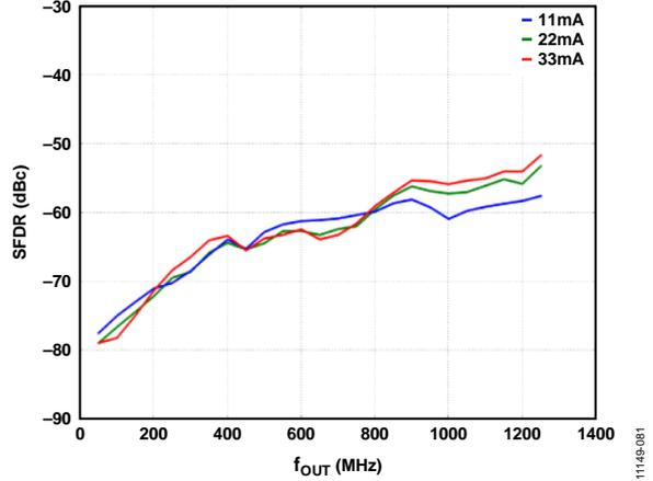
Figure 72. SFDR vs.  $f_{OUT}$  over DAC  $I_{OUTFS}$
