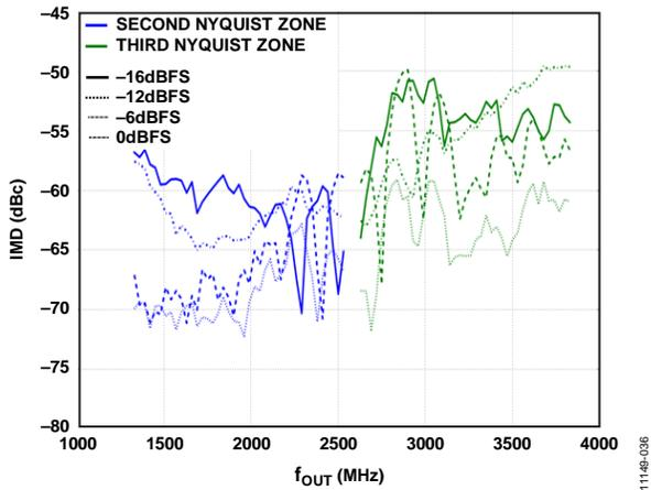
Figure 31. IMD vs.  $f_{OUT}$  over Digital Full Scale
