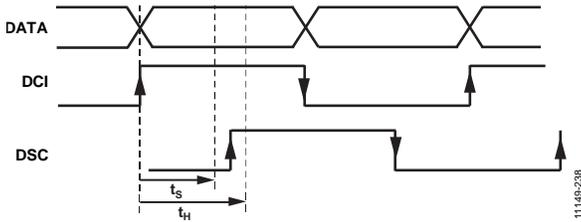
Figure 131. LVDS Data Port Set and Hold Times
