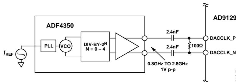
Figure 148. Possible Signal Chain for DACCLK\_x Input
