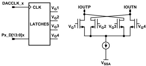
Figure 143. Quad-Switch Architecture
