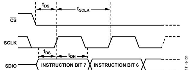
Figure 126. Timing Diagram for an SPI Register Write
