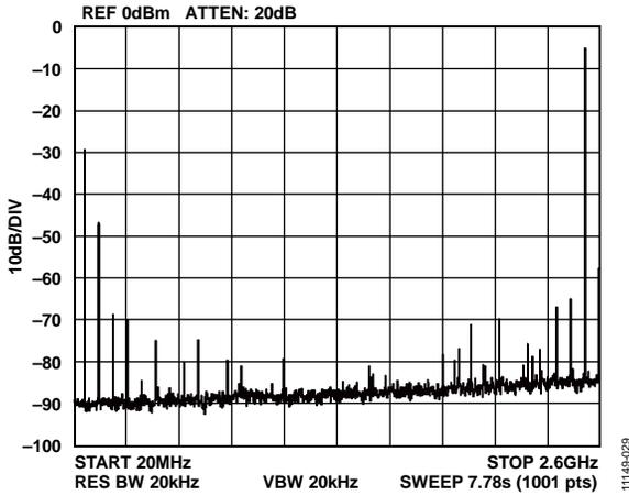
Figure 24. Single Tone Spectrum at  $f_{OUT} = 2350 \text{ MHz}$
