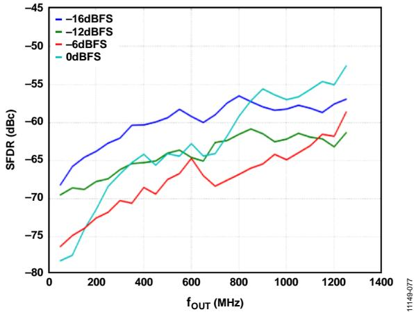
Figure 68. SFDR vs.  $f_{OUT}$  over Digital Full Scale
