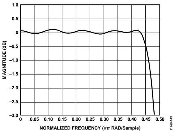
Figure 140. FIR40 2x Interpolation Filter Plot, Pass-Band Ripple
