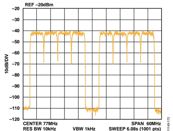
Figure 55. Gap Channel ACPR at 77 MHz
