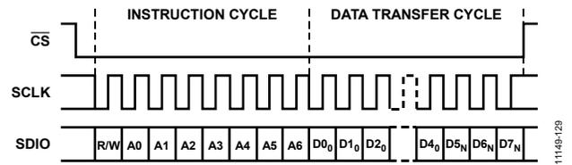
Figure 124. Serial Register Interface Timing, LSB-First Write
