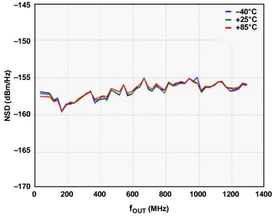
Figure 20. Single-Tone NSD vs.  $f_{OUT}$  over Temperature
