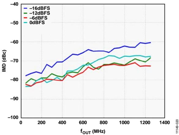
Figure 17. IMD vs.  $f_{OUT}$  over Digital Full Scale
