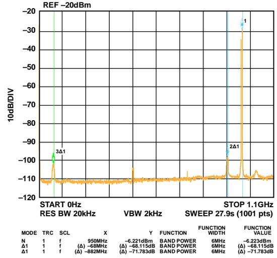
Figure 105. Single Carrier at 950 MHz Output
