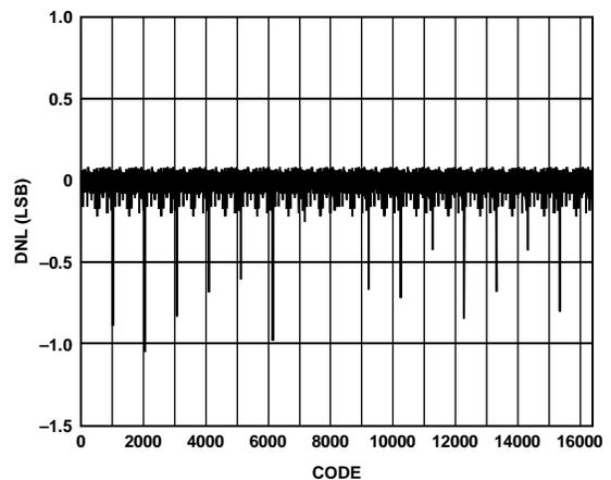
Figure 61. Typical DNL, 33 mA at 25°C
