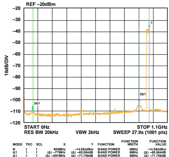
Figure 106. Four Carrier at 950 MHz Output
