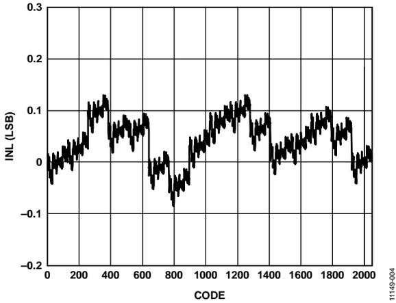
Figure 4. Typical INL, 11 mA at 25°C
