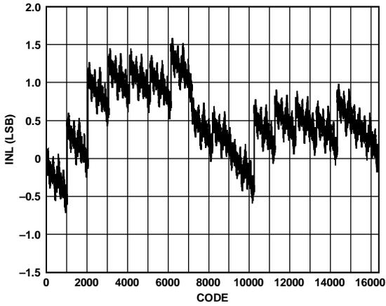
Figure 56. Typical INL, 11 mA at 25°C
