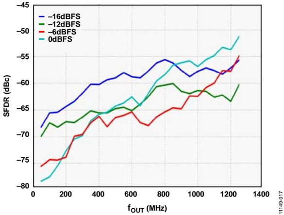
Figure 16. SFDR vs.  $f_{OUT}$  over Digital Full Scale
