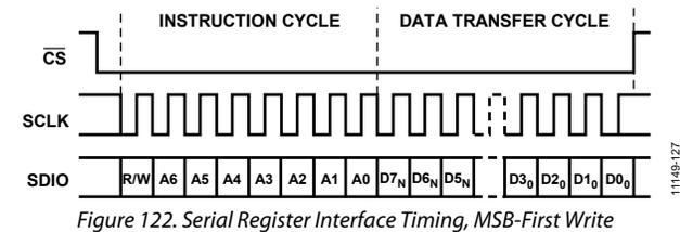
Figure 122. Serial Register Interface Timing, MSB-First Write
