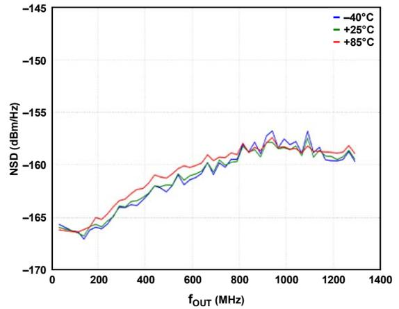
Figure 78. Single-Tone NSD vs.  $f_{OUT}$  over Temperature
