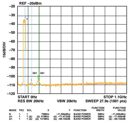
Figure 103. Four Carrier at 70 MHz Output
