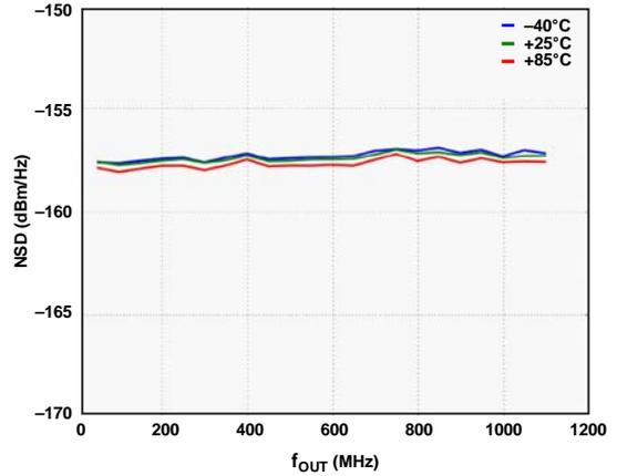
Figure 22. W-CDMA NSD vs.  $f_{OUT}$  over Temperature
