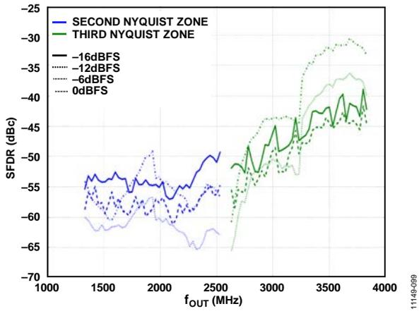
Figure 90. SFDR vs.  $f_{OUT}$  over Digital Full Scale
