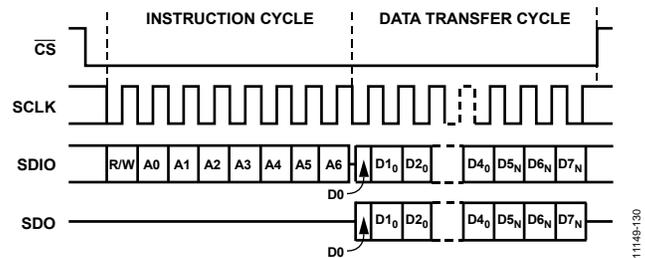
Figure 125. Serial Register Interface Timing, LSB-First Read
