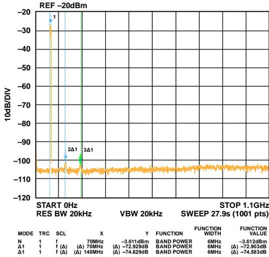
Figure 102. Single Carrier at 70 MHz Output
