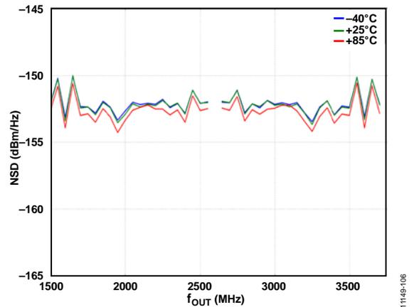
Figure 96. W-CDMA NSD vs.  $f_{OUT}$  over Temperature
