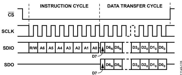
Figure 123. Serial Register Interface Timing, MSB-First Read
