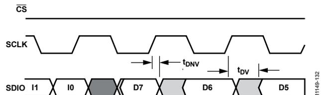
Figure 127. Timing Diagram for an SPI Register Read
