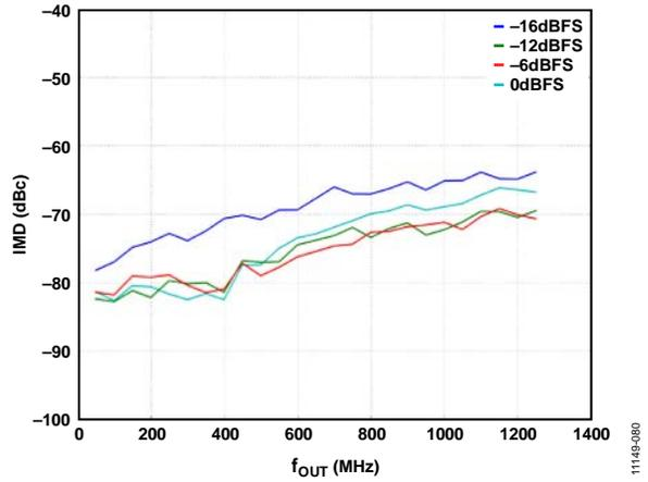
Figure 71. IMD vs.  $f_{OUT}$  over Digital Full Scale
