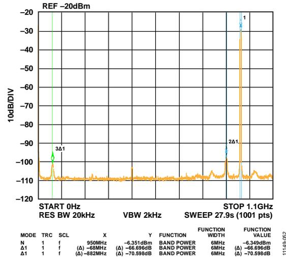
Figure 41. Single Carrier at 950 MHz Output
