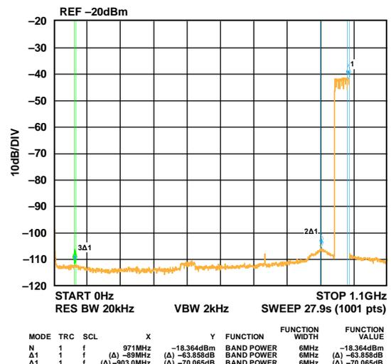
Figure 107. Eight Carrier at 950 MHz Output
