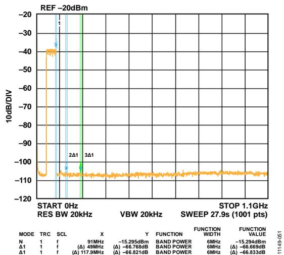
Figure 40. Eight Carrier at 70 MHz Output
