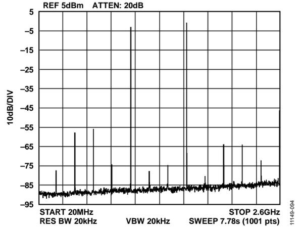
Figure 87. Single-Tone Spectrum at  $f_{OUT} = 1600 \text{ MHz}$
