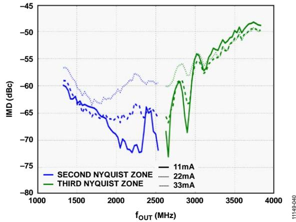
Figure 33. IMD vs.  $f_{OUT}$  over DAC  $I_{OUTFS}$
