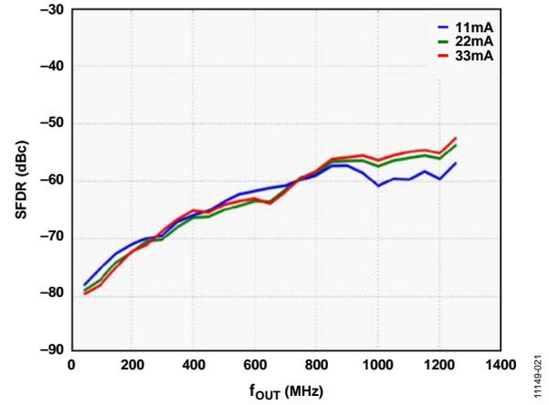
Figure 18. SFDR vs.  $f_{OUT}$  over DAC  $I_{OUTFS}$
