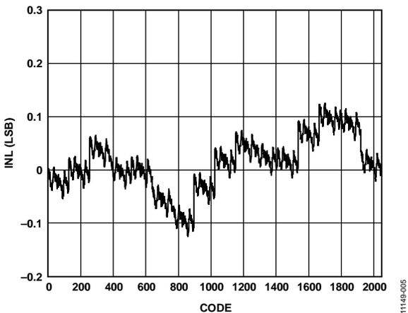
Figure 5. Typical INL, 22 mA at 25°C
