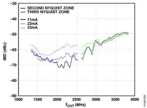
Figure 93. IMD vs.  $f_{OUT}$  over DAC  $I_{OUTFS}$
