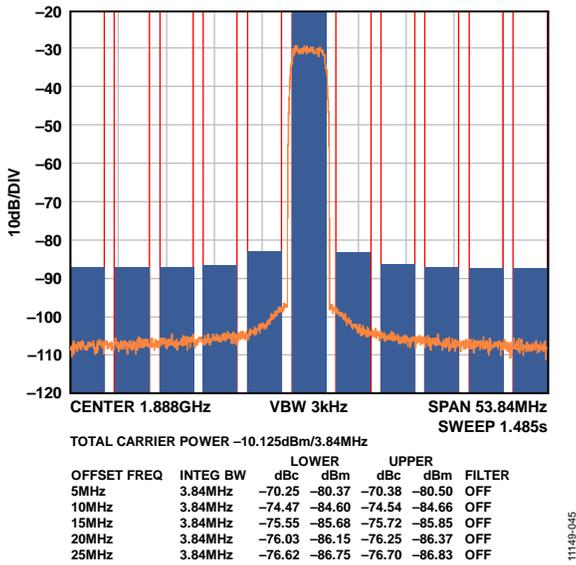
Figure 35. Single-Carrier W-CDMA at 1887.5 MHz
