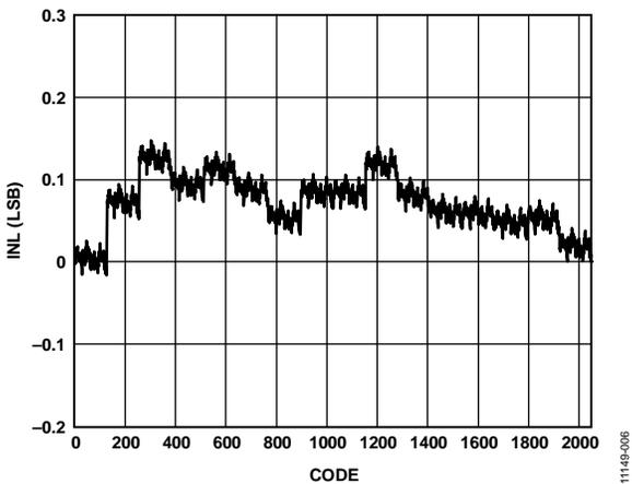
Figure 6. Typical INL, 33 mA at 25°C
