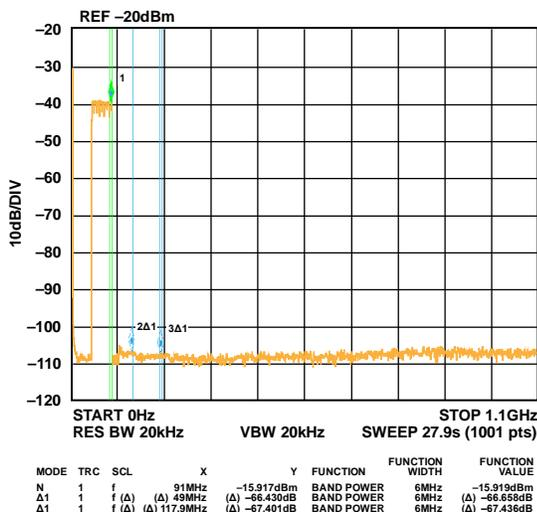
Figure 104. Eight Carrier at 70 MHz Output
