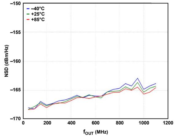
Figure 77. W-CDMA NSD vs.  $f_{OUT}$  over Temperature
