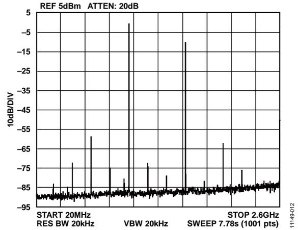
Figure 13. Single-Tone Spectrum at  $f_{OUT} = 1000 \text{ MHz}$
