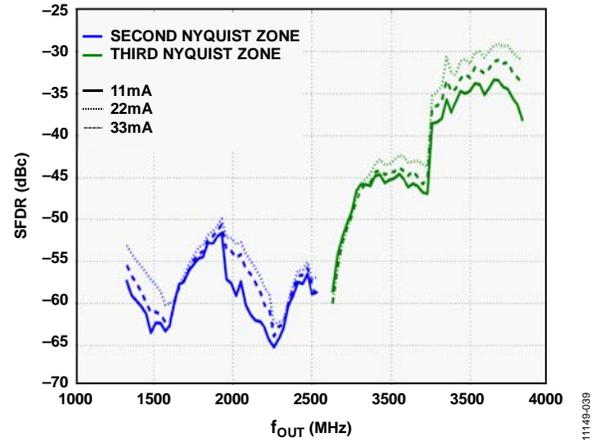
Figure 32. SFDR vs.  $f_{OUT}$  over DAC  $I_{OUTFS}$
