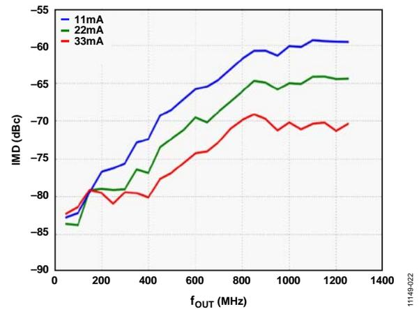
Figure 19. IMD vs.  $f_{OUT}$  over DAC  $I_{OUTFS}$
