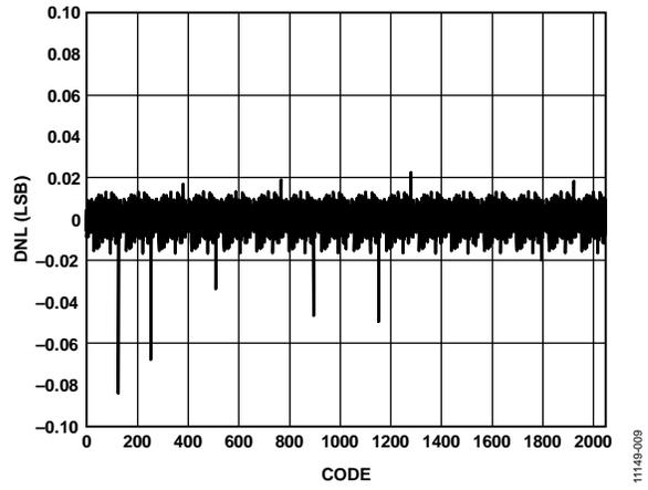
Figure 9. Typical DNL, 33 mA at 25°C
