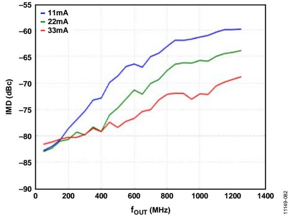
Figure 73. IMD vs.  $f_{OUT}$  over DAC  $I_{OUTFS}$
