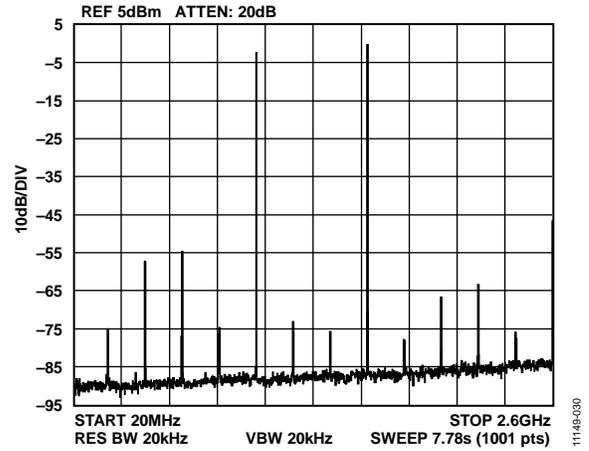
Figure 27. Single-Tone Spectrum at  $f_{OUT} = 1600 \text{ MHz}$
