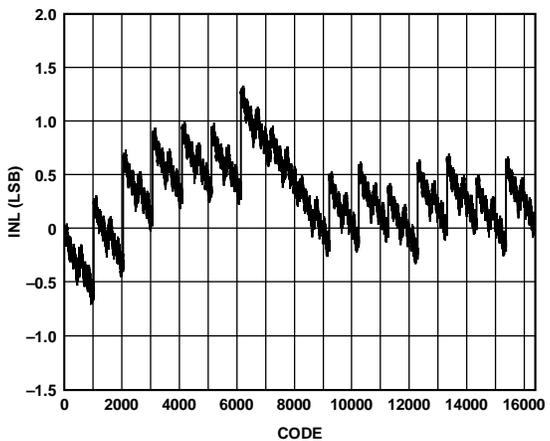
Figure 58. Typical INL, 33 mA at 25°C
