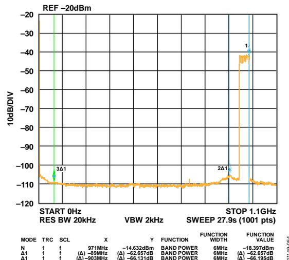
Figure 43. Eight Carrier at 950 MHz Output
