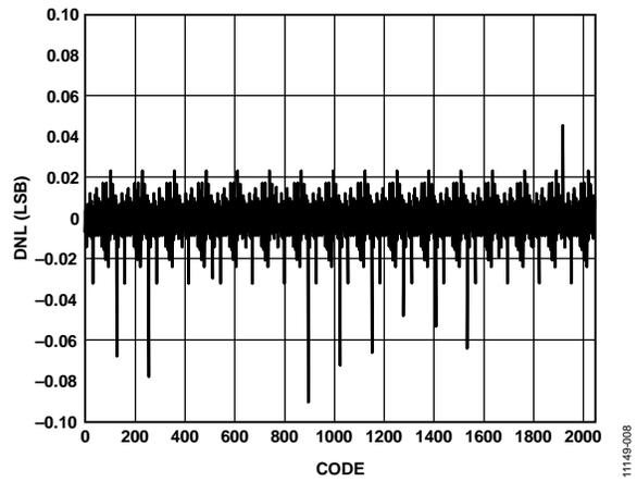
Figure 8. Typical DNL, 22 mA at 25°C
