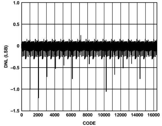
Figure 59. Typical DNL, 11 mA at 25°C
