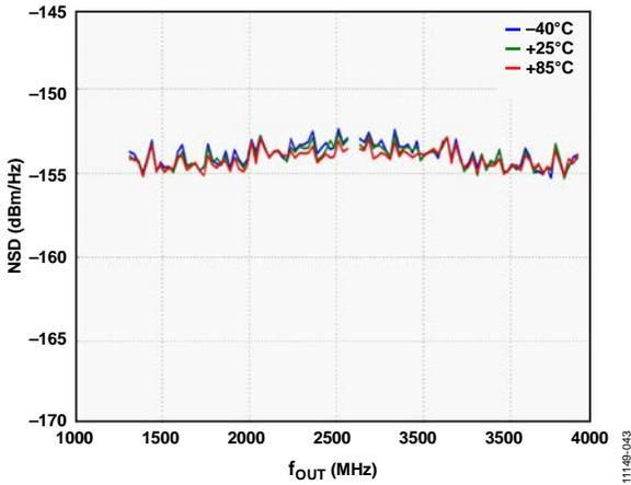
Figure 34. Single-Tone NSD vs.  $f_{OUT}$  over Temperature
