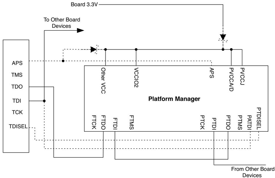
Figure 51. Power Manager PTDI/PATDI Pin Selection Diagram
