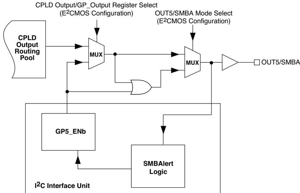
The typical flow for an SMBAAlert transaction is as follows (Figure 38):
