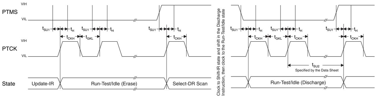
Figure 8. Programming Timing Diagram
