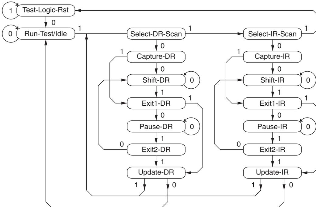
Note: The value shown adjacent to each state transition in this figure represents the signal present at PTMS at the time of a rising edge at PTCK.
