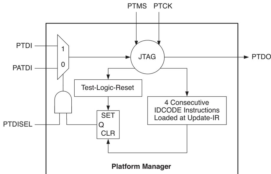
Table 21 shows in truth table form the same conditions required to select either PTDI or PATDI as in the logic diagram found in Figure 50.
