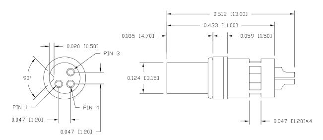
ΝΠΤΕ: MATERIAL HOUSING: TPU, BLACK SHELL: BRASS BRASS CONTACT: NUT: BRASS □-RING: NBR, BLACK FINISH TIN PLATED SHELL: CONTACT: GOLD PLATED OVER 504 NICKEL NICKEL PLATED NUT: ELECTRICAL RATED CURRENT: 1A RATED VOLTAGE: 60V INSULATION RESISTANCE: 100 MΩ MIN. CONTACT RESISTANCE: 10 m $\Omega$  MAX. IP67 WATER PROOF: ENVIRONMENT **OPERATION TEMPERATURE:** -40°C TD +85°C WIRE GAUGE: 28 AWG MAX RECOMMENDED
