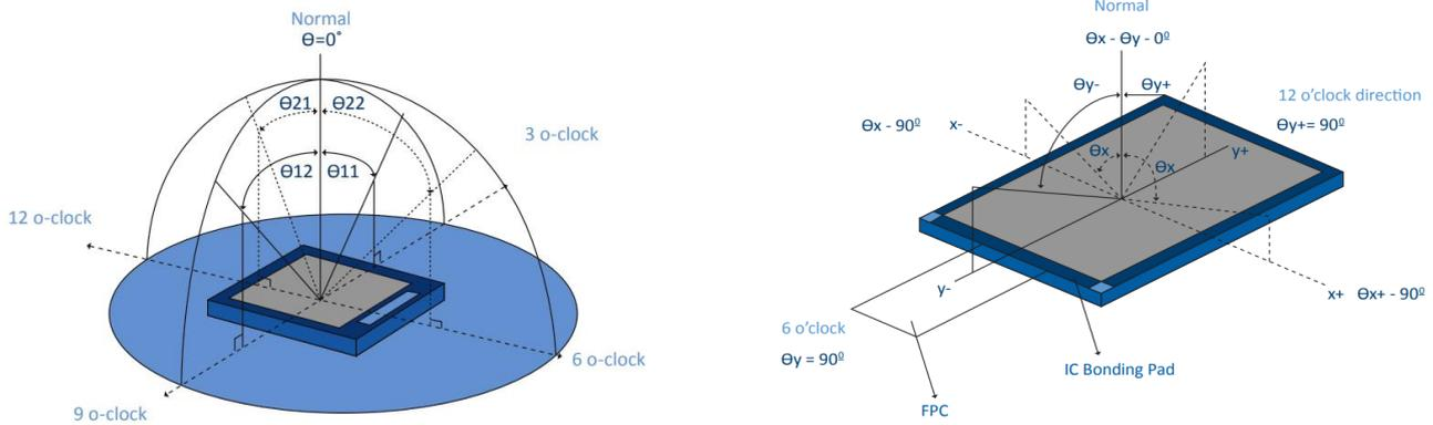
(2) Definition of Contrast Ratio (Cr): measured at the center point of panel. The contrast ratio (Cr) measured on a module, is the ratio between the luminance (Lw) in a full white area (R=G=B=1) and the luminance (Ld) in a dark area (R=G=B=0).
