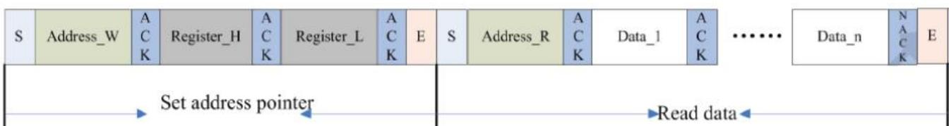
The host issues the start condition once again and sends 0xBB (read operation). After receiving ACK, the host starts to read the data. GT9271 also supports continuous read operation. When receiving a byte of data, the host sends an ACK signal indicating successful reception. After receiving the last byte of data, the host sends a NACK signal followed by a STOP condition which terminates communication.
