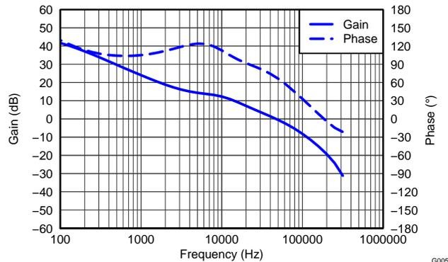
Figure 24. CLOSED LOOP RESPONSE, VIN = 5 V, IOUT = 1.5 A
