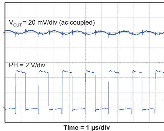
Figure 30. OUTPUT VOLTAGE RIPPLE,  $I_{OUT} = 3\text{ A}$
