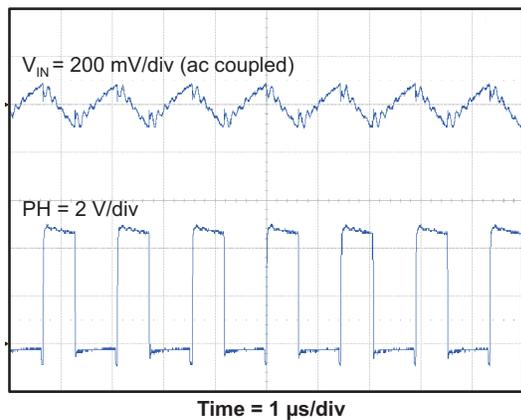
Figure 29. INPUT VOLTAGE RIPPLE,  $I_{OUT} = 3\text{ A}$
