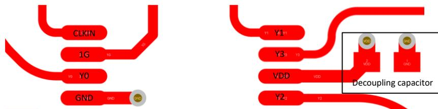
Figure 12-1. PCB Conceptual Layout
