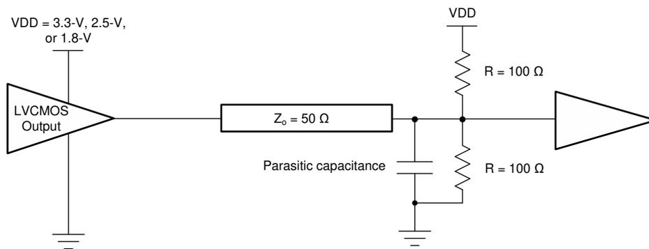
**Figure 8-2. Application Load With 50-ohm Termination**
