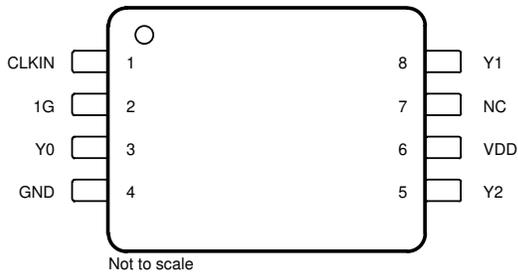
Figure 6-3. LMK1C1103 PW Package 8-Pin TSSOP Top View
