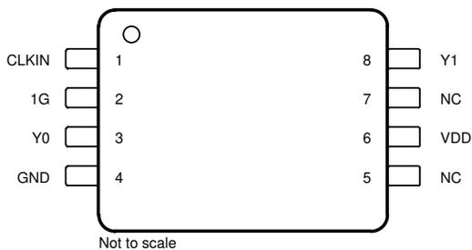
Figure 6-1. LMK1C1102 PW Package 8-Pin TSSOP Top View
