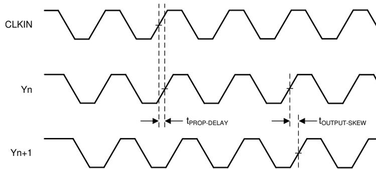
**Figure 8-6. Propagation Delay  $t_{PROP-DELAY}$  and Output Skew  $t_{OUTPUT-SKEW}$**
