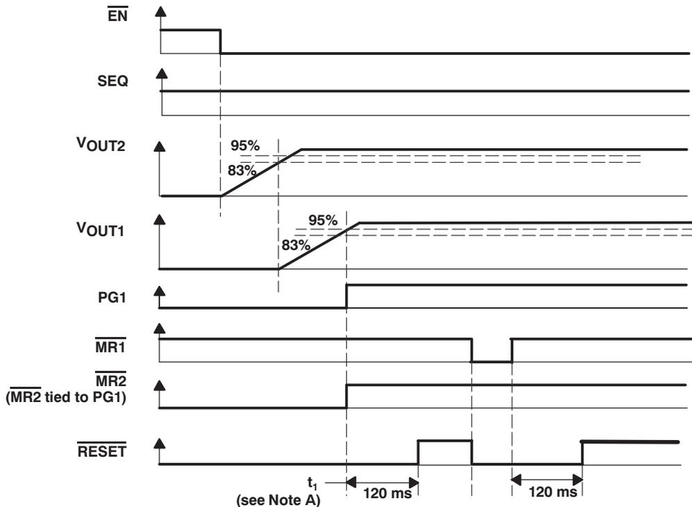
NOTE A:  $t_1$ : Time at which both  $V_{OUT1}$  and  $V_{OUT2}$  are greater than the PG thresholds and MR1 is logic high.
