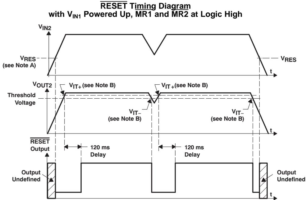
NOTES: A.  $V_{RES}$  is the minimum input voltage for a valid  $\overline{\text{RESET}}$ . The symbol  $V_{RES}$  is not currently listed within EIA or JEDEC standards for semiconductor symbology.
