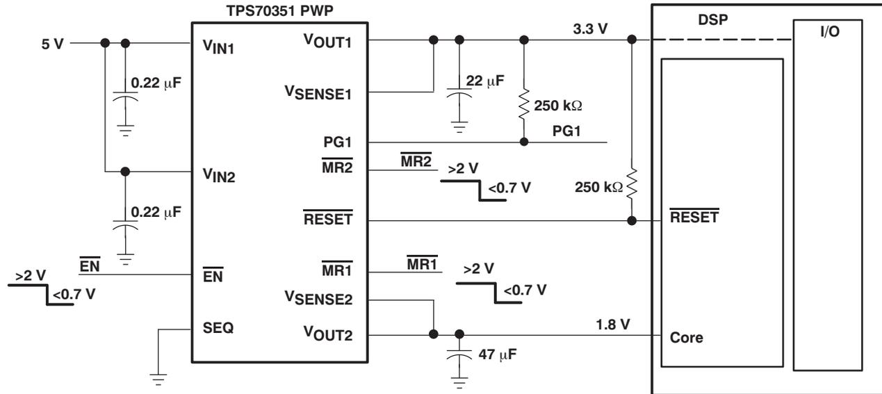
The TPS703xx family of voltage regulators offers very low dropout voltage and dual outputs with power up sequence control, designed primarily for DSP applications. These devices have low noise output performance without using any added filter bypass capacitors, and are designed to have a fast transient response and be stable with 47  $\mu$ F low ESR capacitors.
