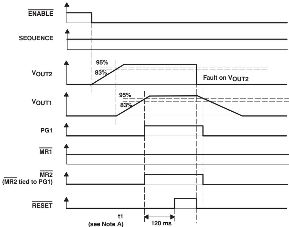
NOTE A:  $t_1$ : Time at which both  $V_{OUT1}$  and  $V_{OUT2}$  are greater than the PG thresholds and MR1 is logic high.
