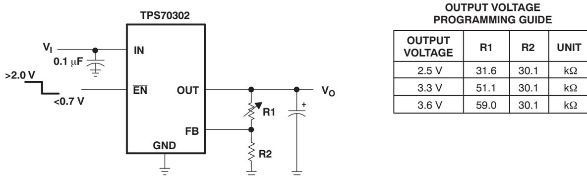
Figure 45. TPS70302 Adjustable LDO Regulator Programming
