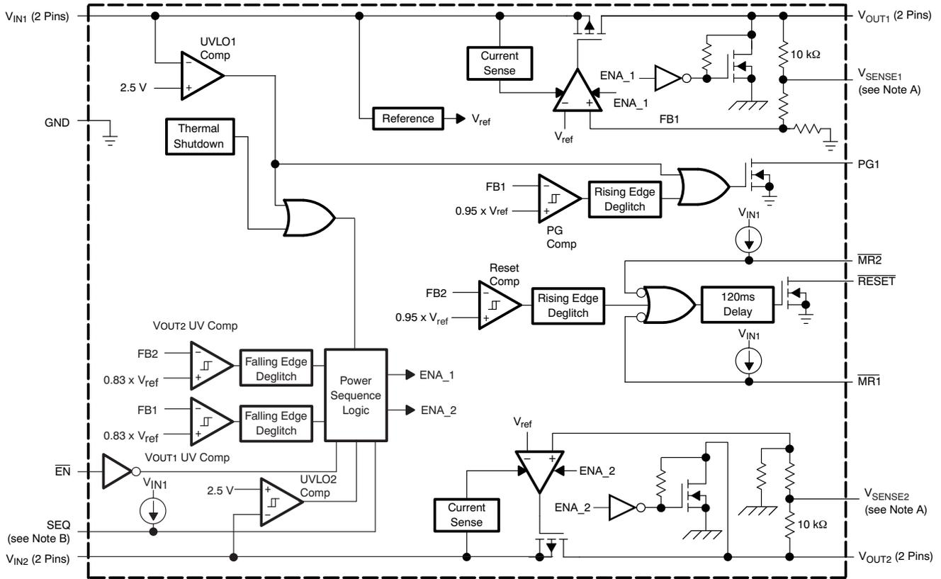
A. For most applications, FB1 and FB2 should be externally connected to resistor dividers as close as possible to the device. For other implementations, refer to FB terminals connection discussion in the [Application Information](#) section.
