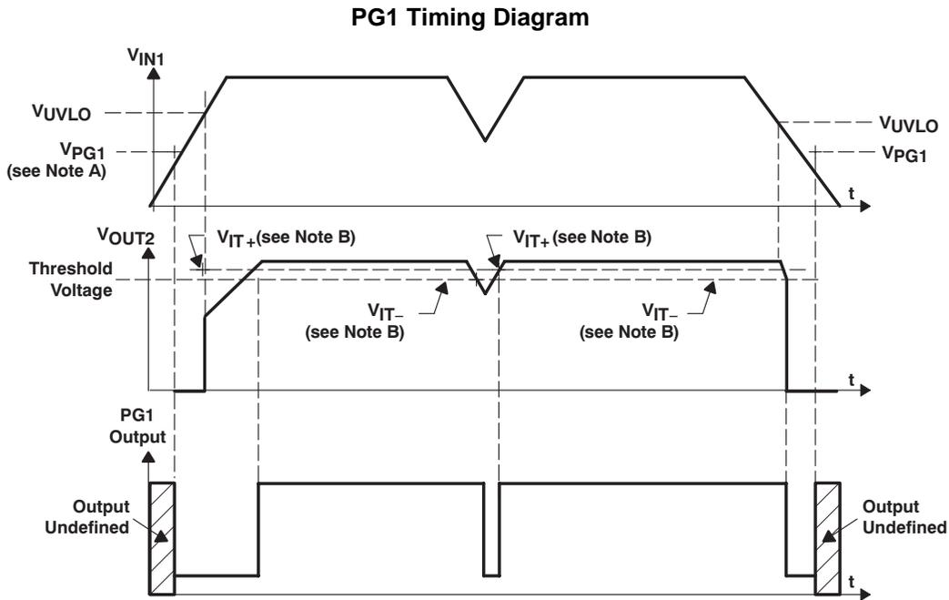
NOTES: A.  $V_{PG1}$  is the minimum input voltage for a valid PG1. The symbol  $V_{PG1}$  is not currently listed within EIA or JEDEC standards for semiconductor symbology.
