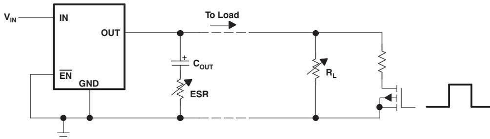
Figure 28. Test Circuit for Typical Regions of Stability
