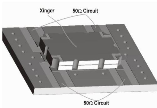
**Figure 3: Component Placement**
