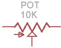
Of course, we've just learned so much about using resistors to adjust the current going through an LED, we can use the knob of the potentiometer as a physical way to control the LED.
