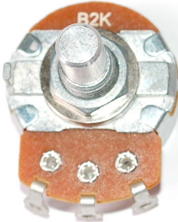
Potentiometers, like resistors, have an Ohm value. For example, this potetiometer is a **2Kohm** (its printed up top). Potentiometers have three pins, two 'outer' and one 'middle' pin. The middle pin is sometimes called the wiper.
