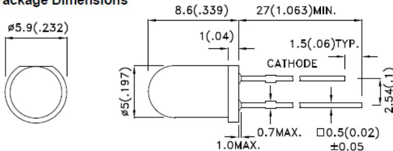
As you can see, the main diameter of the LED is 5mm (its a '5mm LED') and there's a lip that makes it around 6mm. The lip can make it handy if you're gluing the LED into a drilled hole, so it doesnt fall through. The datasheet also tells you which pin is the cathode and other lengths and sizes. Note that the figures are in mm with the inches in ()'s afterwards.
