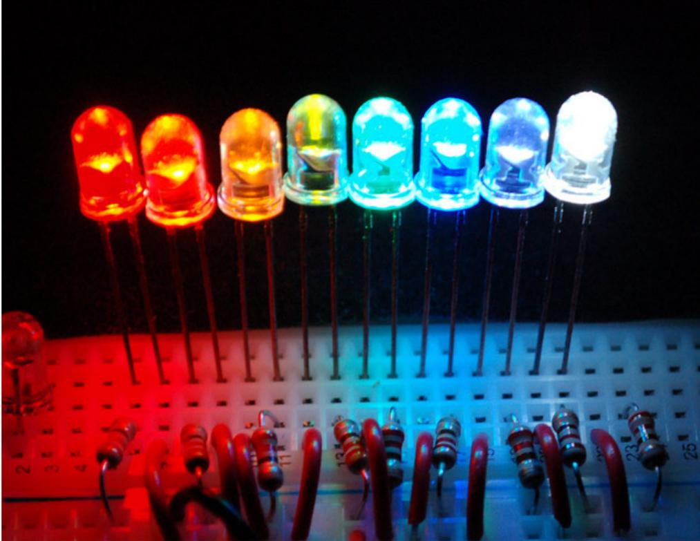
This tutorial will cover those wonderful blinky things, LEDs. We're going to cover how to calculate the current going through an LED and in the mean time introduce two important laws of electronics, **Kirchhoff's Voltage Law** and **Ohm's Law**. We'll begin by performing experiments that will demonstrate how voltage and resistance affects current and then prove those results with a little math.
