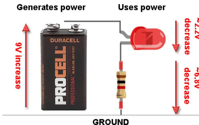
Whenever the LED is on, the voltage it uses it up is somewhere between 1.85V and 2.5V. We'll say 2.2V for average - that's a good assumption for most red, yellow, orange and light-green LEDs. If we subtract that from 9V we get about 6.8V left. This is the voltage that must be 'absorbed' by the resistor.
