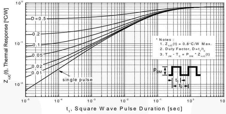
Figure 11-2. Transient Thermal Response Curve for FQPF10N60C
