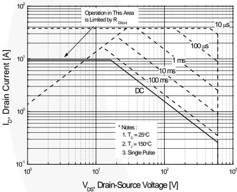
**Figure 9-2. Maximum Safe Operating Area for FQPF10N60C**
