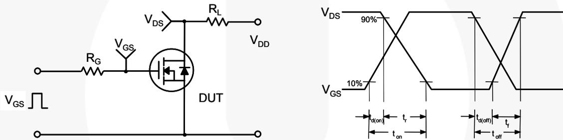
Figure 13. Resistive Switching Test Circuit & Waveforms
