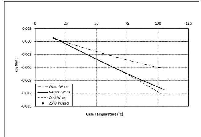
**Figure 9: Typical DC ccx Shift vs. Case Temperature**
