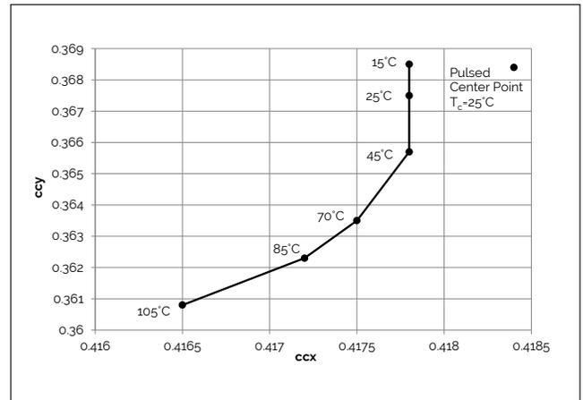
**Figure 15: 3500K Class A Color Shift vs. Case Temperature<sup>1</sup>**
