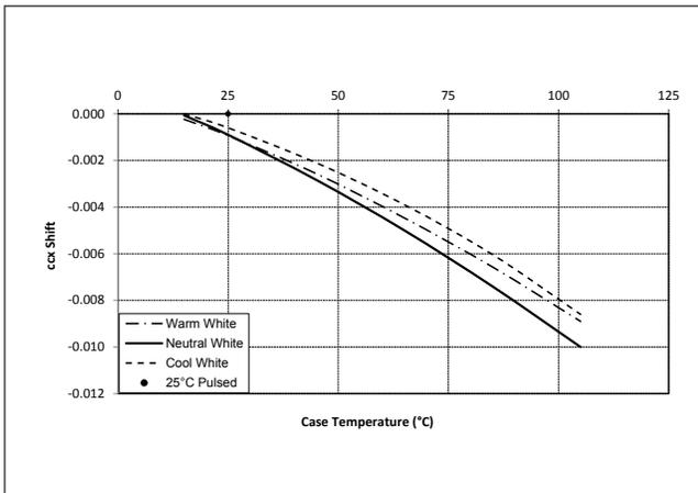
**Figure 10: 2000K, 65 CRI Color Shift vs. Case Temperature**
