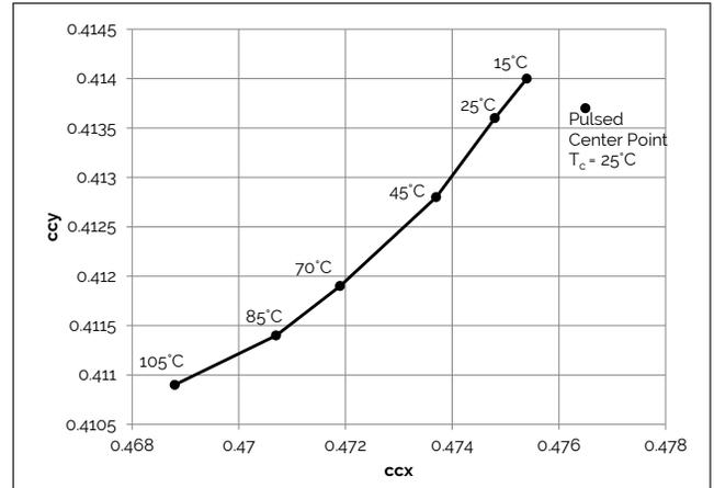
**Figure 13: 5600K Color Shift vs. Case Temperature<sup>1,3</sup>**
