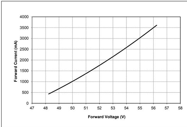
**Figure 2: Vero SE 29C Drive Current vs. Voltage**
