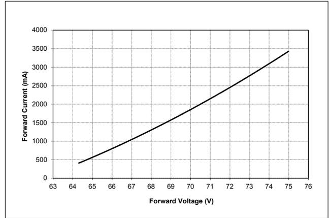
**Figure 3: Vero SE 29D Drive Current vs. Voltage**
