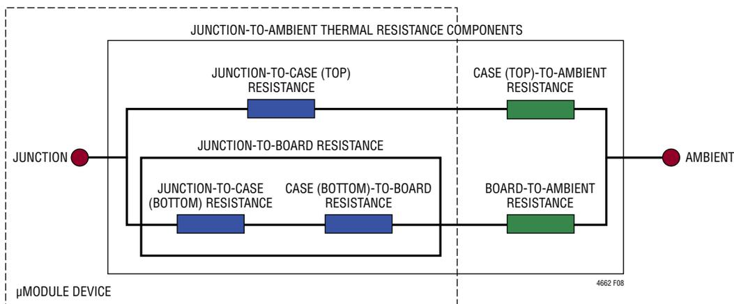
Figure 8. Graphical Representation of JESD51-12 Thermal Coefficients
