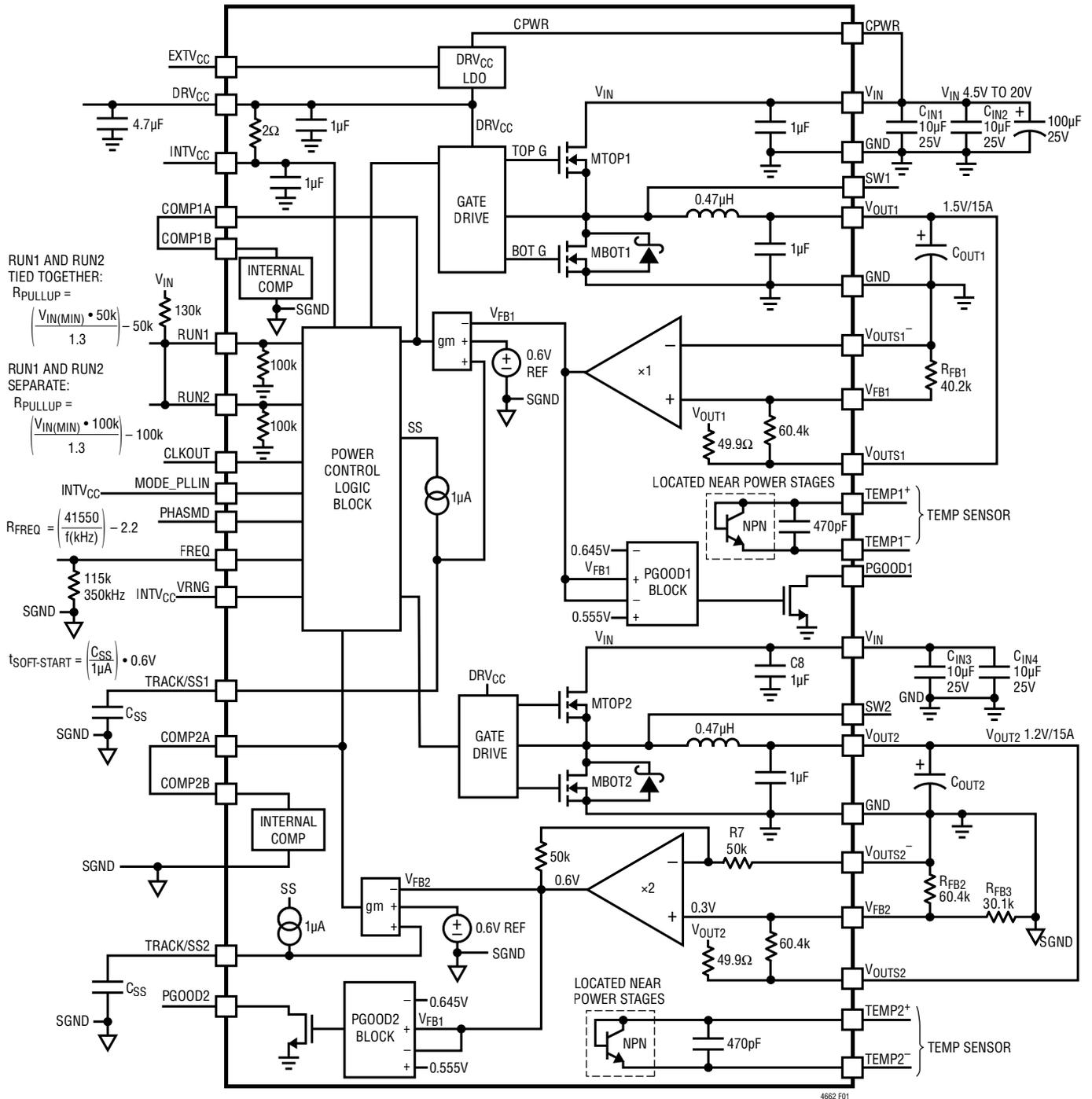
Figure 1. Simplified LTM4662 Block Diagram
