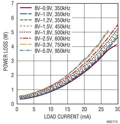
Figure 12. 8V<sub>IN</sub> Power Loss Curve
