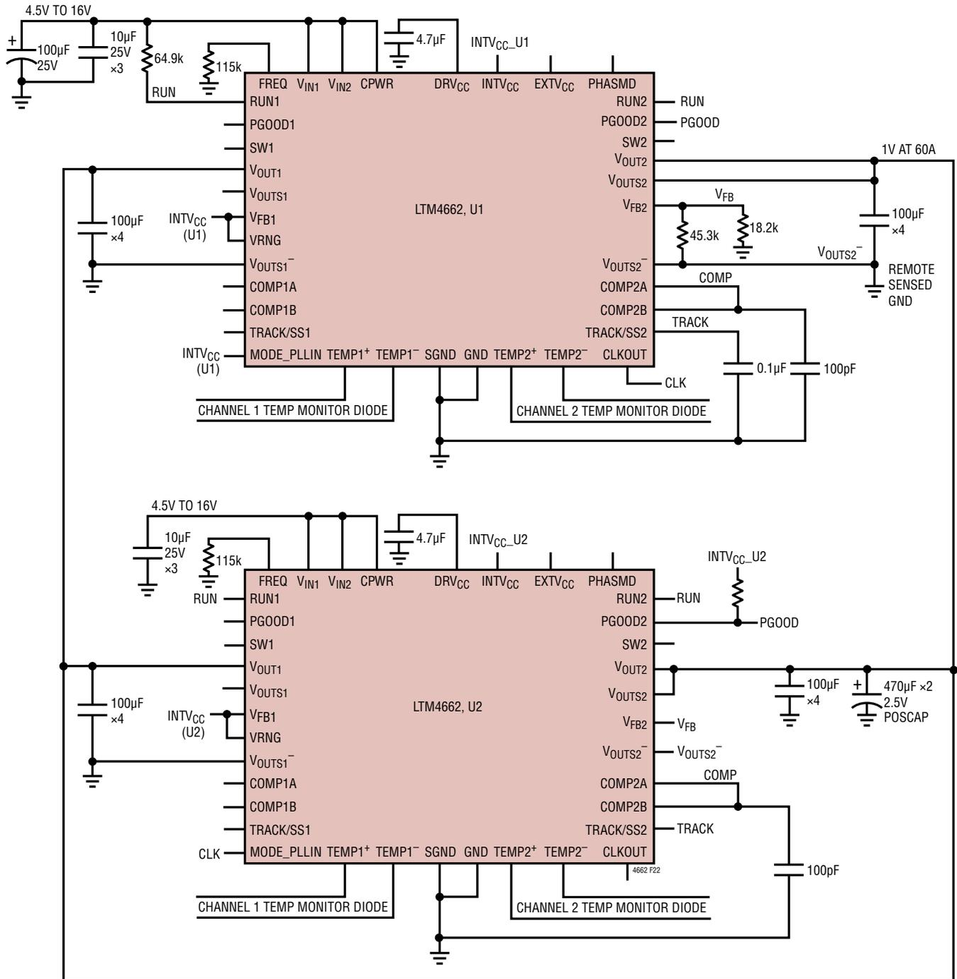
Figure 22. Four Phase Design 1V at 60A
