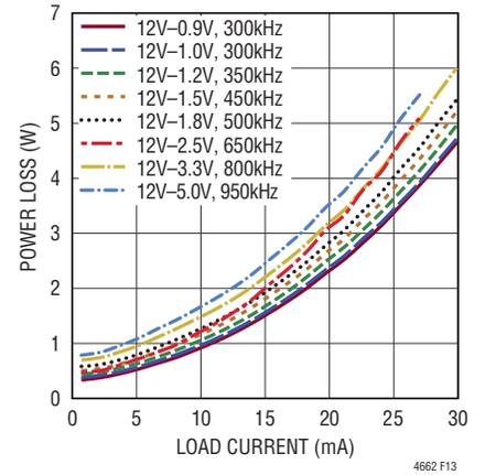
Figure 13. 12V<sub>IN</sub> Power Loss Curve
