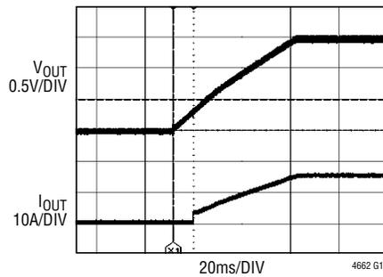
$12V_{IN}$ ,  $1.5V_{OUT}$  AT 15A LOAD
