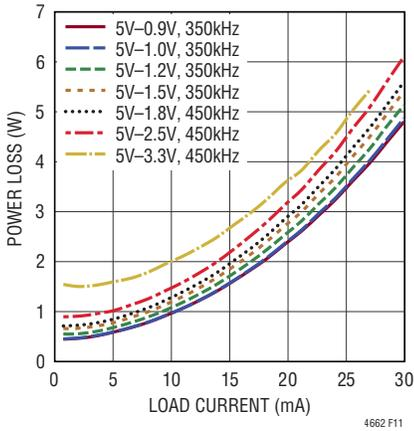
Figure 11. 5V<sub>IN</sub> Power Loss Curve
