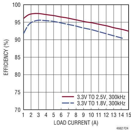
Figure 24. Efficiency, 3.3V<sub>IN</sub>
