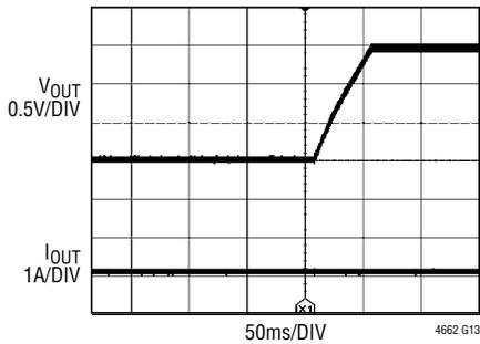
$12V_{IN}$ ,  $1.5V_{OUT}$  AT NO LOAD
