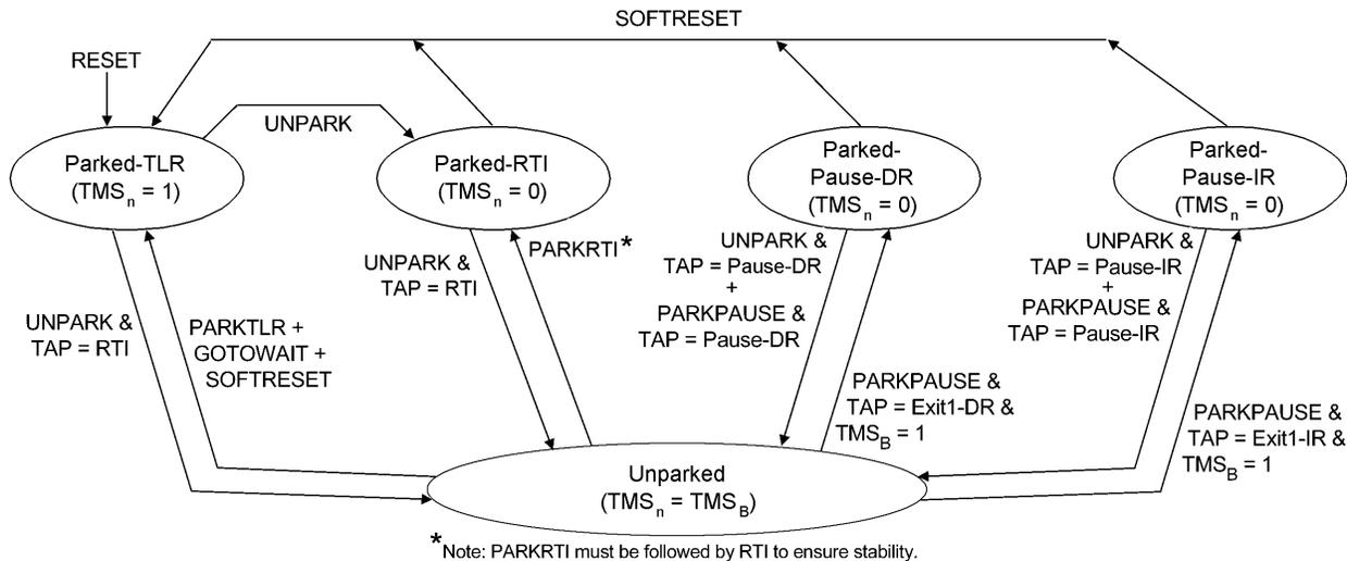
**Figure 4. Local SCANSTA111 Port Configuration State Machine**
