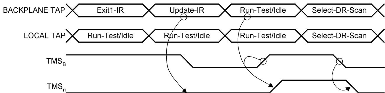
Figure 10. Local Scan Port Synchronization from Parked-RTI State
