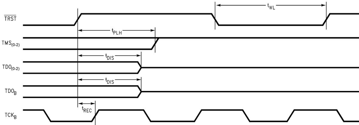
Figure 16. Reset Waveforms
