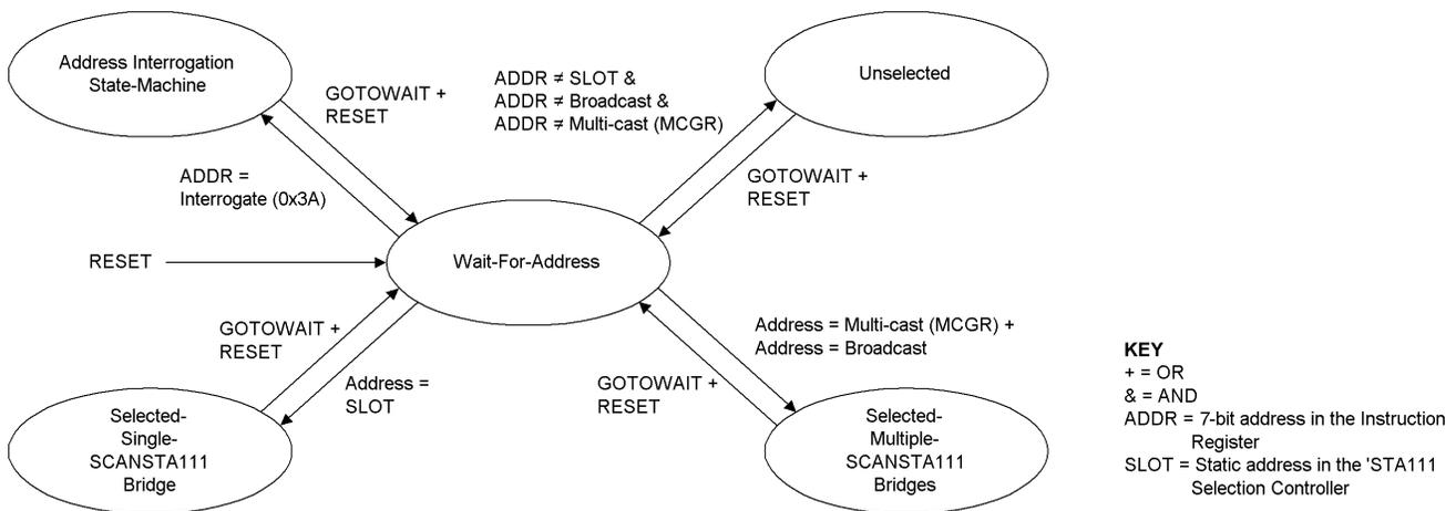
**Figure 3. State Machine for SCANSTA111 Selection Controller**
