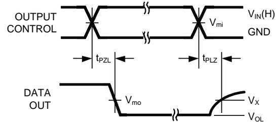
**Figure 21. TRI-STATE Output Low Enable and Disable Times for Logic**
