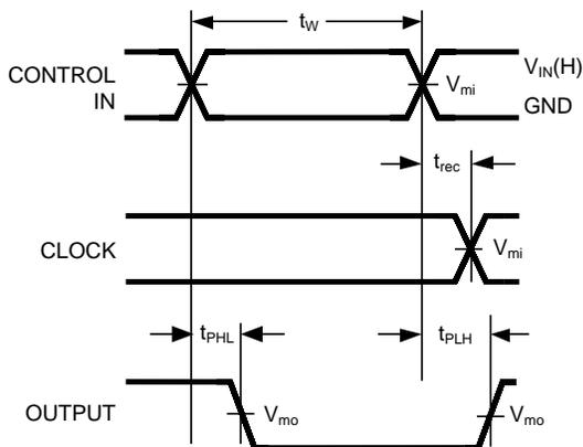
**Figure 20. Propagation Delay, Pulse Width and  $t_{REC}$  Waveforms**
