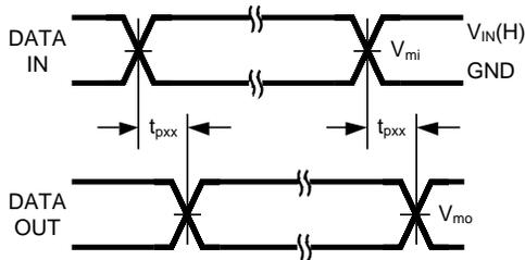
**Figure 18. Waveform for Inverting and Non-inverting Functions**
