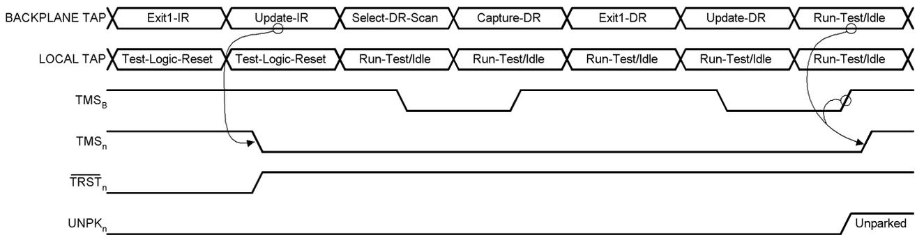
Figure 11. Local Scan Port Synchronization on Second Pass
