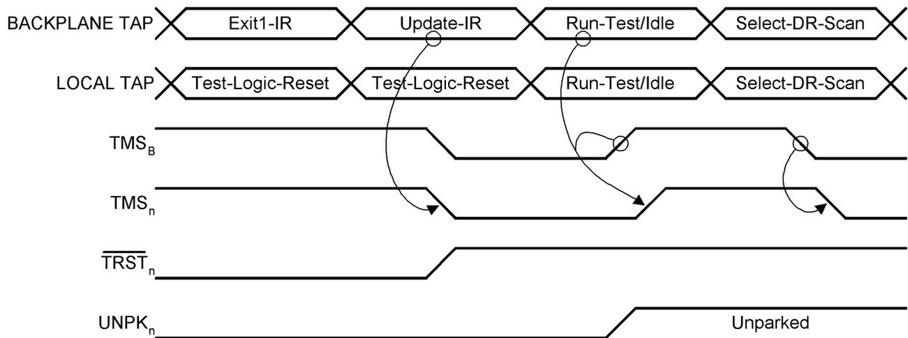
Figure 9. Local Scan Port Synchronization from Parked-TLR State
