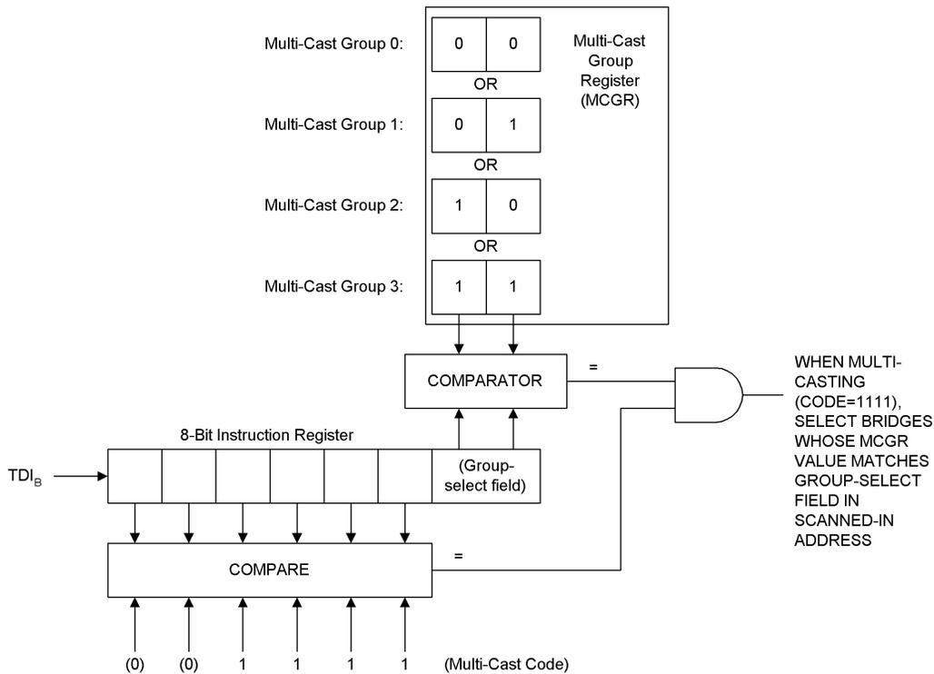
Figure 8. Multi-Cast Addressing: Address Loaded into Instruction Register
