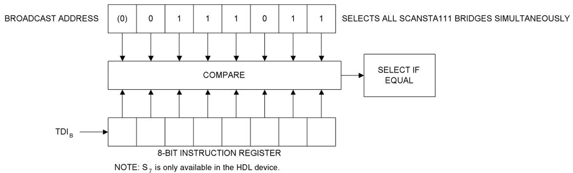
Figure 7. Broadcast Addressing: Address Loaded into Instruction Register
