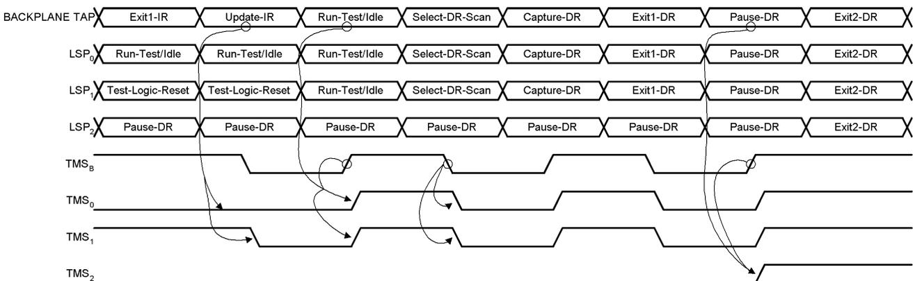
Figure 12. Synchronization of the Three Local Scan Ports
