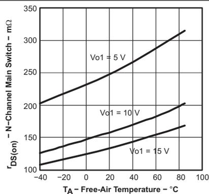
Figure 2.  $r_{DS(on)}$  N-Channel Main Switch vs Free-Air Temperature
