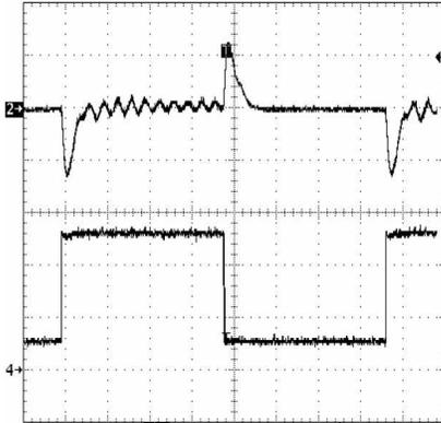
**Figure 9. Overcompensated (Damped Oscillation),  $R_C$  is Too Large**
