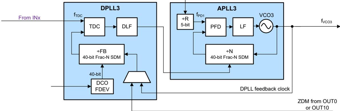
**Figure 8-6. APLL Cascaded With DPLLs Disabled Example**
