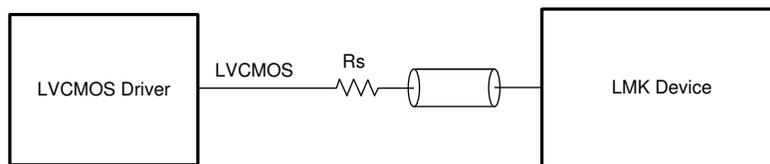
**Figure 8-10. Single-Ended LVC MOS (1.8 V, 2.5 V, 3.3 V) to Reference (IN<sub>x</sub>\_P) or XO Input (XO)**
