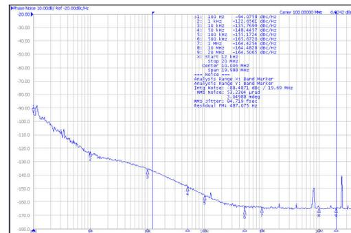
Jitter = 85 fs RMS (12 kHz to 20 MHz)
