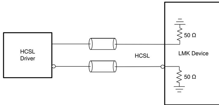
**Figure 8-13. HCSL (Load Terminated) to Reference (INx)**
