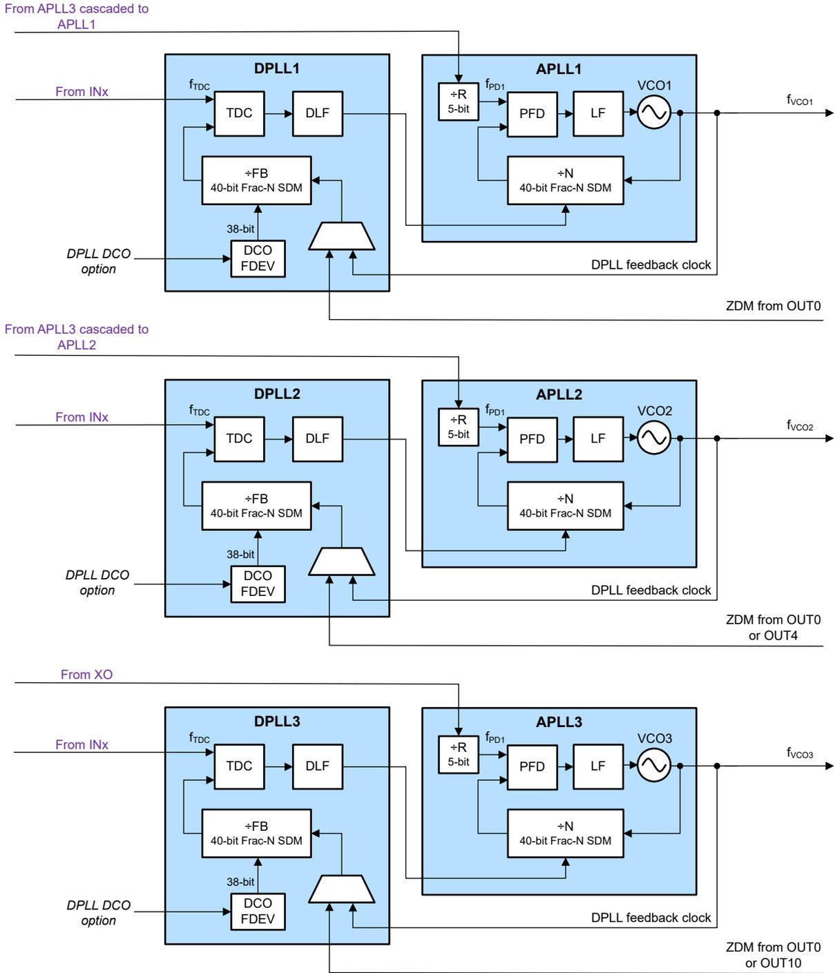
**Figure 8-5. APLL Cascaded With DPLLs Enabled Example**
