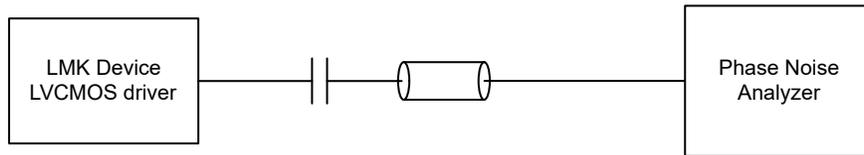
**Figure 7-4. LVC MOS Output Phase Domain Test Configuration**
