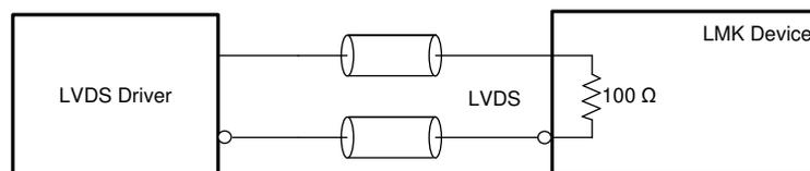
**Figure 8-12. DC-Coupled HSDS/LVDS to Reference (IN<sub>x</sub>)**
