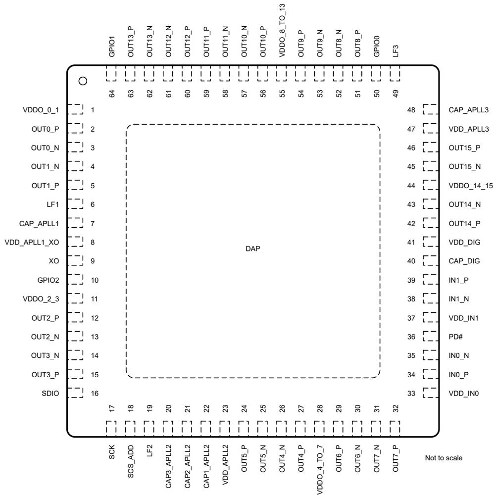
Figure 5-1. LMK5B33216 RGC Package 64-Pin VQFN Top View
