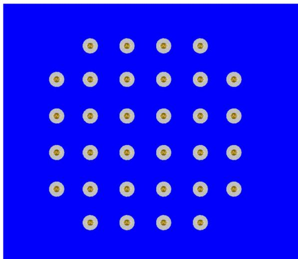
Figure 9-19. PCB Layout Example for LMK5B33216, Bottom Layer
