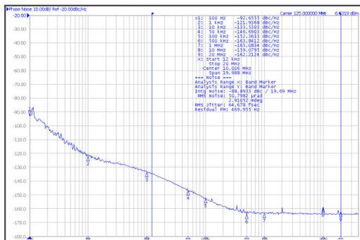
Jitter = 65 fs RMS (12 kHz to 20 MHz)
