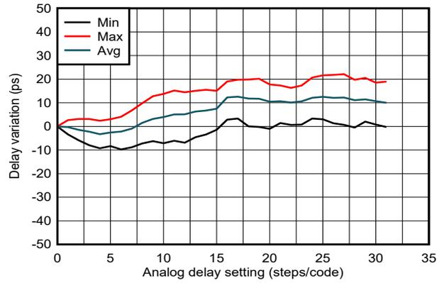
**Figure 6-11. SYSREF/1-PPS Delay Linearity vs Analog Delay Code 5**
