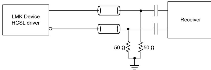
**Figure 8-28. AC-Coupled HCSL Output Termination**
