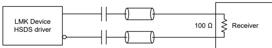
Figure 8-25. AC-Coupled HSDS Output Termination Method 1
