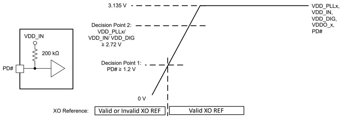
Figure 9-1. Recommendation for Power Up From a Single-Supply Rail
