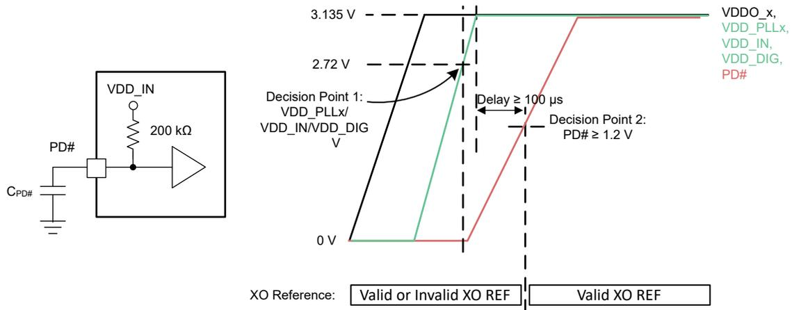
**Figure 9-2. Recommendation for Power Up From Split-Supply Rails**
