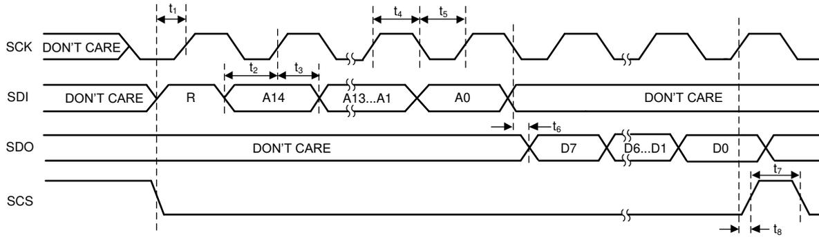
**Figure 6-2. SPI 4-Wire Read Timing Diagram**
