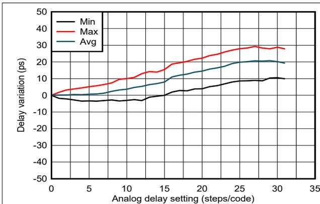
Figure 6-8. SYSREF/1-PPS Delay Linearity vs Analog Delay Code 2
