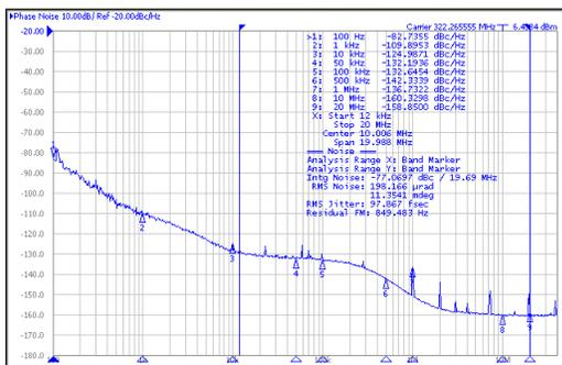
Jitter = 97 fs RMS (12 kHz to 20 MHz)
