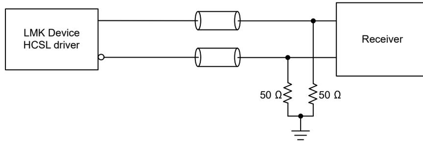
**Figure 8-27. DC-Coupled HCSL Output Termination**
