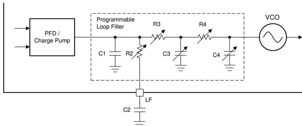
**Figure 8-22. Loop Filter Structure of Each APLL**
