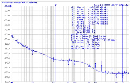
Jitter = 103 fs RMS (12 kHz to 20 MHz)
