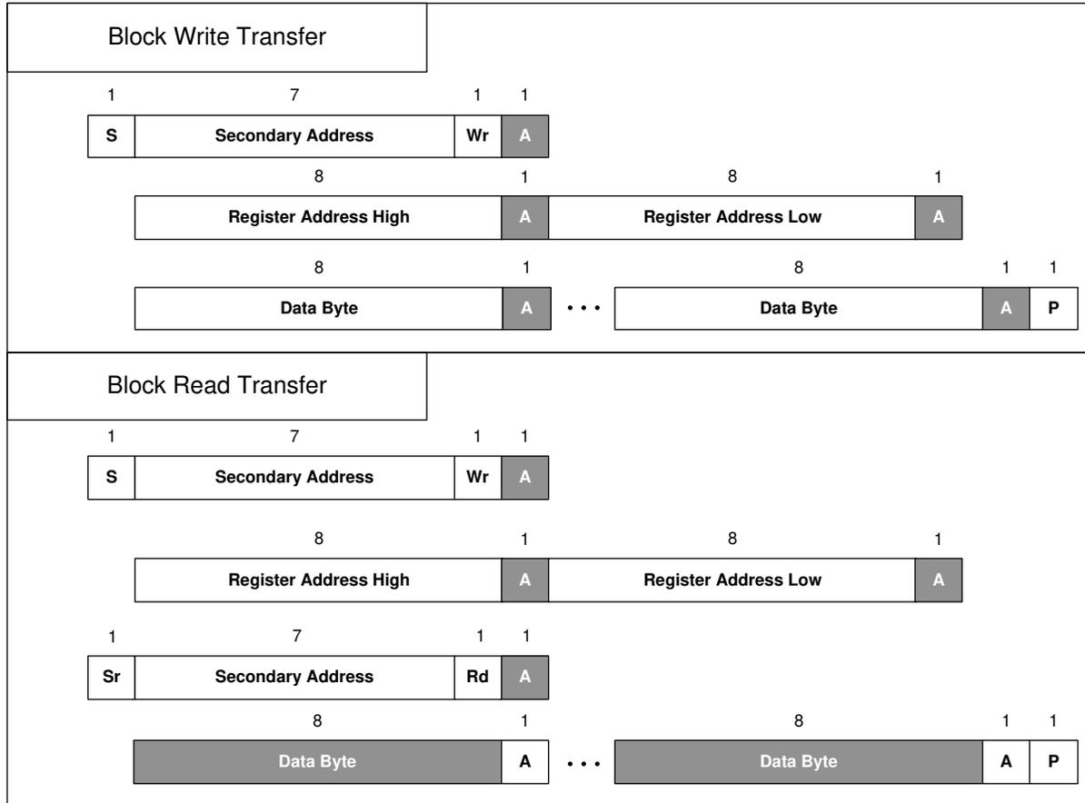
Figure 8-41. I<sup>2</sup>C Block Register Transfers
