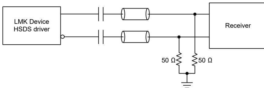
Figure 8-26. AC-Coupled HSDS Output Termination Method 2
