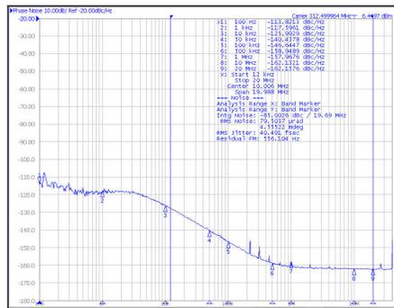
Jitter = 41 fs RMS (12 kHz to 20 MHz)
