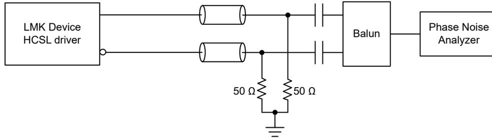
**Figure 7-8. HCSL Output Time Domain Test Configuration**
