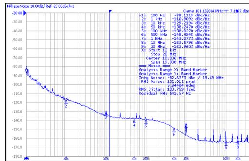
Jitter = 105 fs RMS (12 kHz to 20 MHz)
