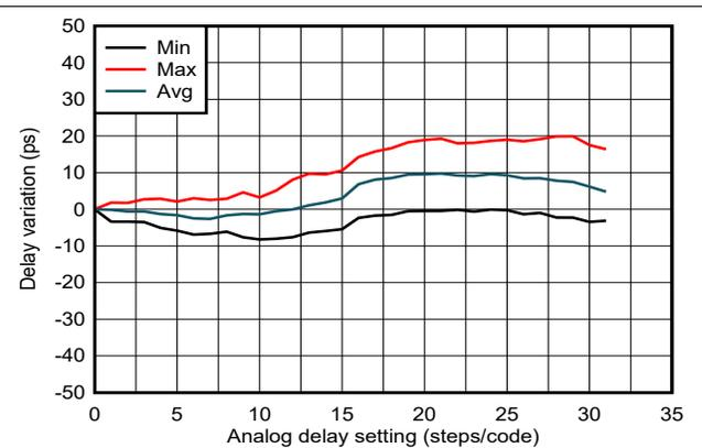
Figure 6-9. SYSREF/1-PPS Delay Linearity vs Analog Delay Code 3
