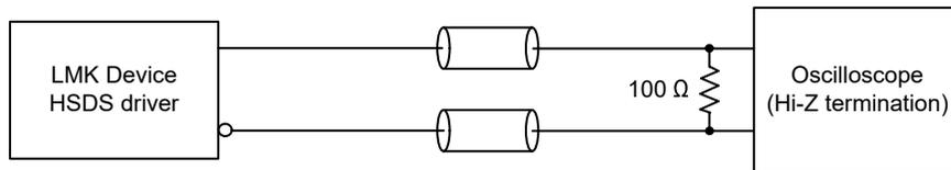
**Figure 7-5. HSDS Output Time Domain Test Configuration**
