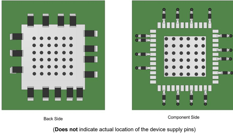
**Figure 9-17. Generalized Placement of Power Supply Bypass Capacitors**
