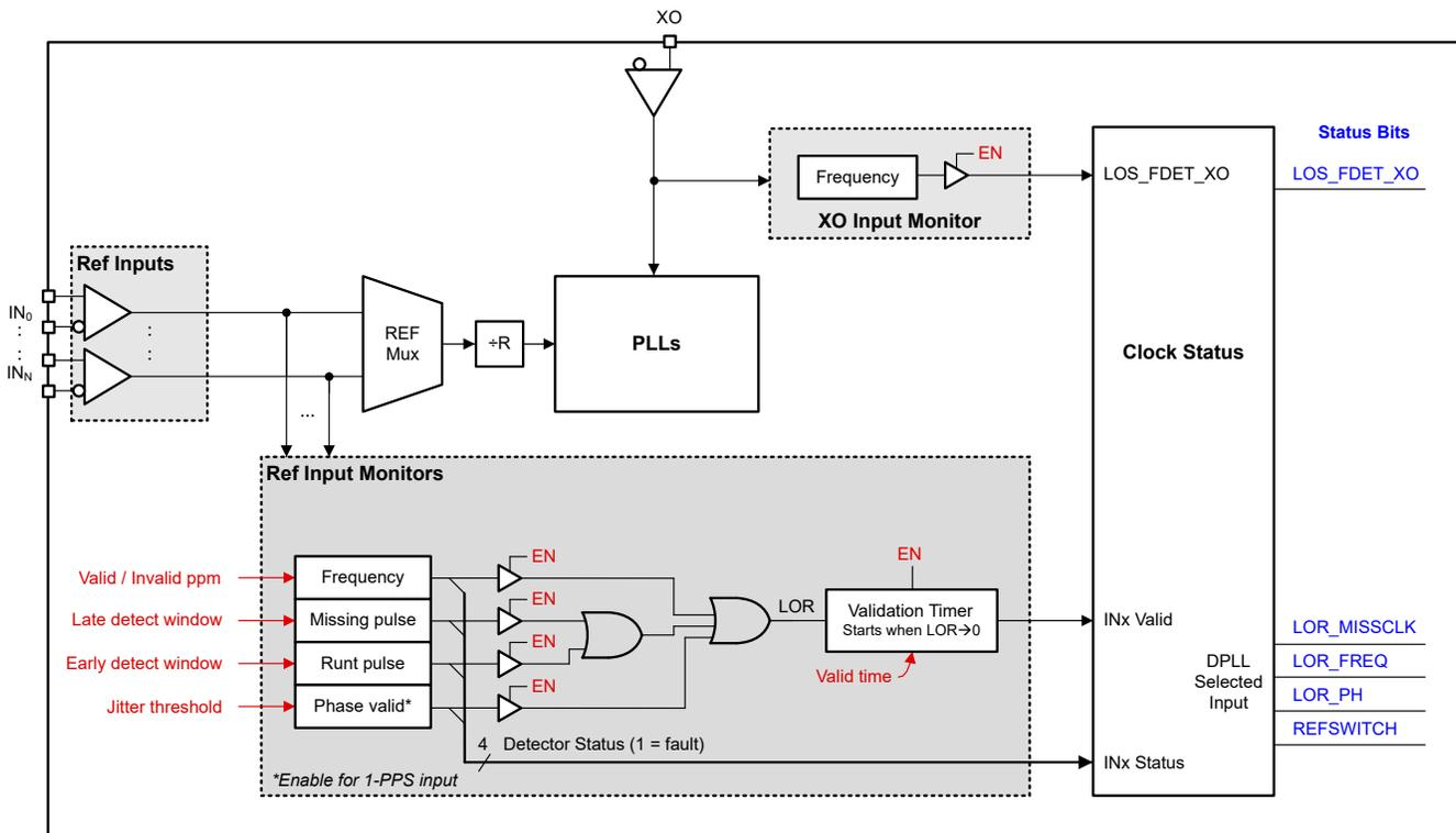
Figure 8-15. Clock Monitors for Reference and XO Inputs
