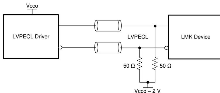
**Figure 8-11. DC-Coupled LVPECL to Reference (IN<sub>x</sub>)**
