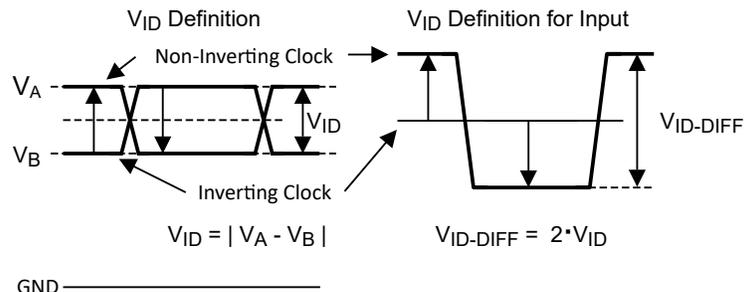
**Figure 7-1. Two Different Definitions for Differential Input Signals**
