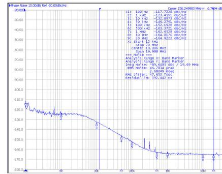
Jitter = 47 fs RMS (12 kHz to 20 MHz)
