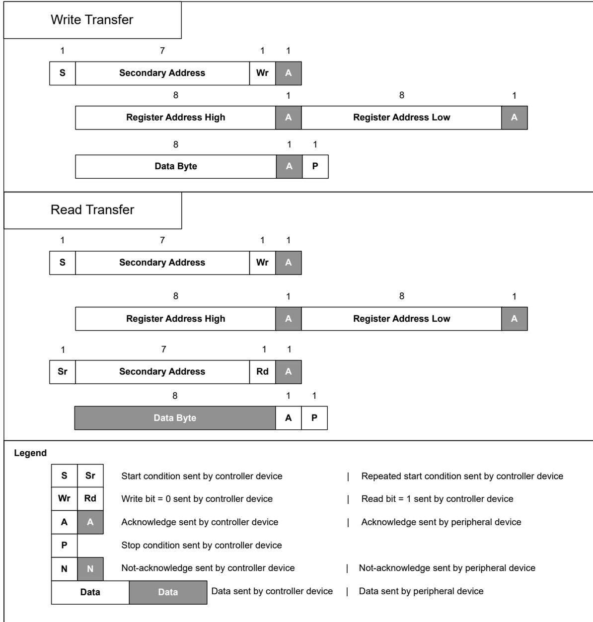
**Figure 8-40. I<sup>2</sup>C Byte Write and Read Transfers**
