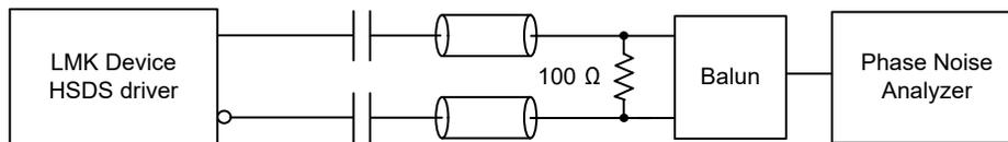
**Figure 7-6. HSDS Output Phase Domain Test Configuration**
