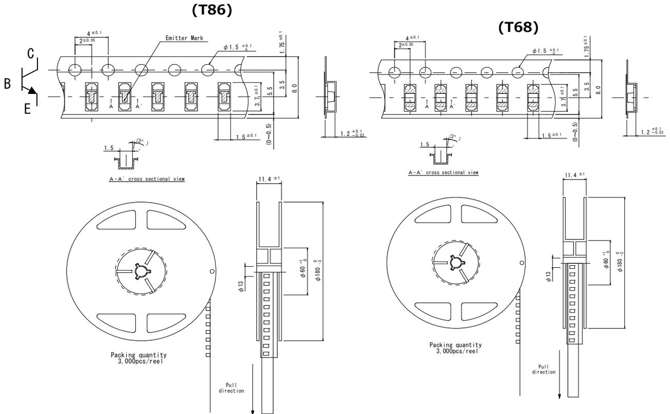
Note) Tolerance is within ±0.2mm unless otherwise specified.
