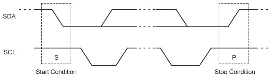
**Figure 8-3. Definition Of Start And Stop Conditions**
