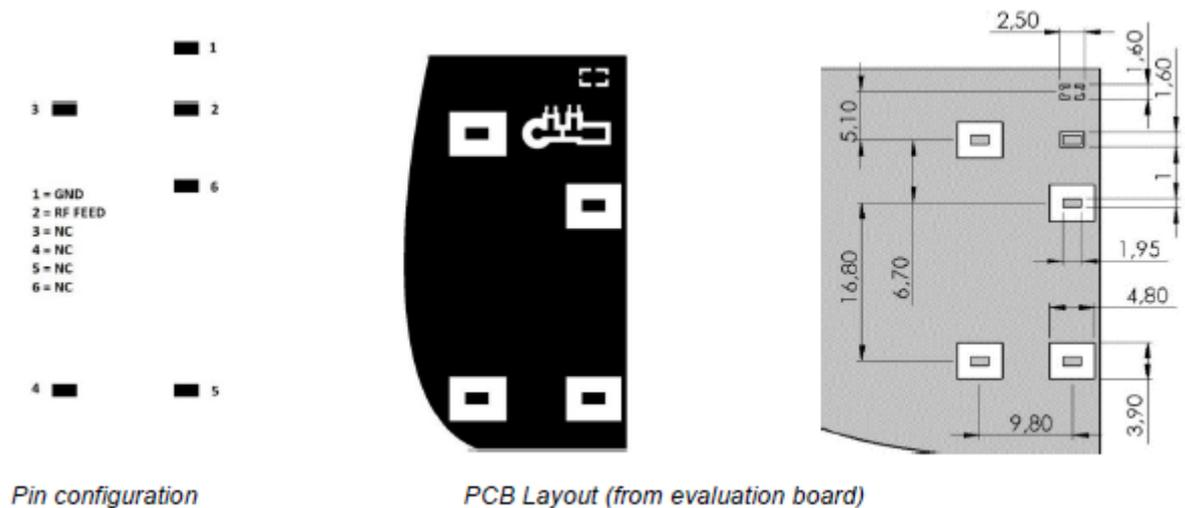
The antenna is preferably positioned along one side of the PCB ground plane, where pin 1 shall be as close as possible to the layout corner.
