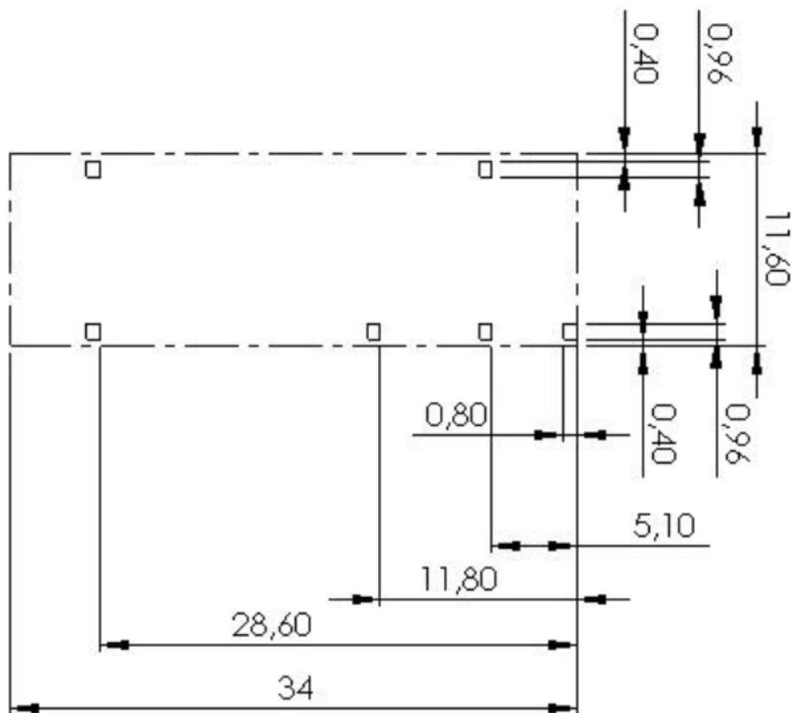
The sketch shows the antenna footprint and keep-out block. Above dimensions are mm.
